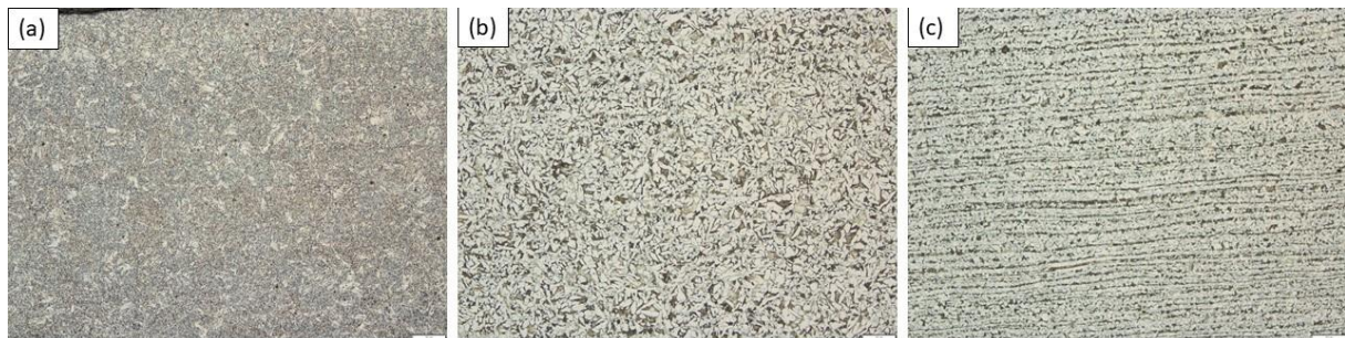
Figure 3-13: Microstructure gradient of Steel Grade B for water quenched tube blank, 500x, scale: 20 \mu m
