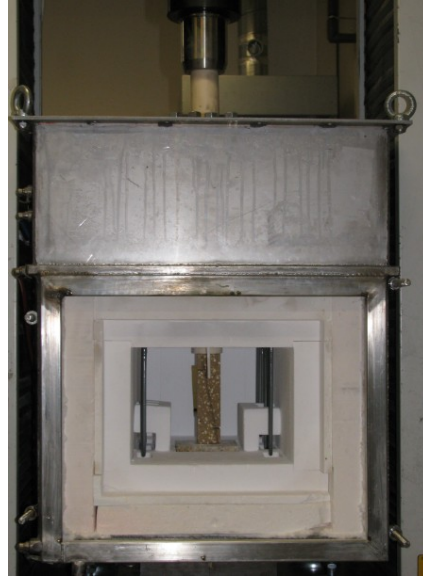
Figure II-18: Uniaxial compression test at elevated temperature.
