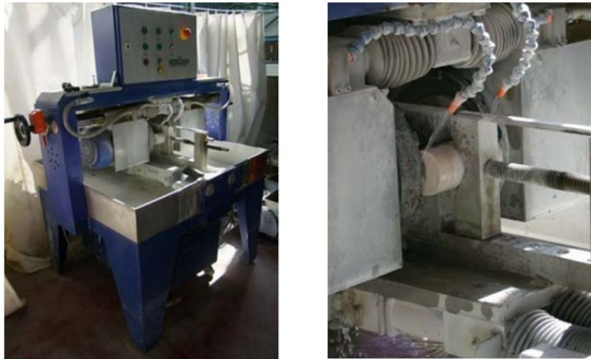
Figure II-27: Plan milling machine for producing specimens with parallel endfaces.
