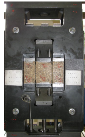
Figure II-5: Double direct shear test.
