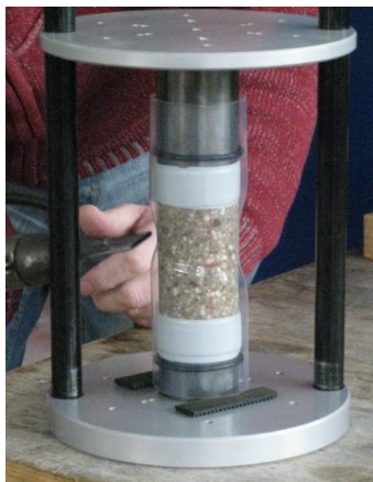
Figure II-28: Sample preparation. Heating the polyolefin tube on the sample to provide an impermeable barrier to confining pressure.
