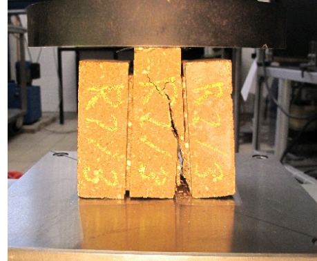
Figure II-3: Fracture of the double direct shear test.
