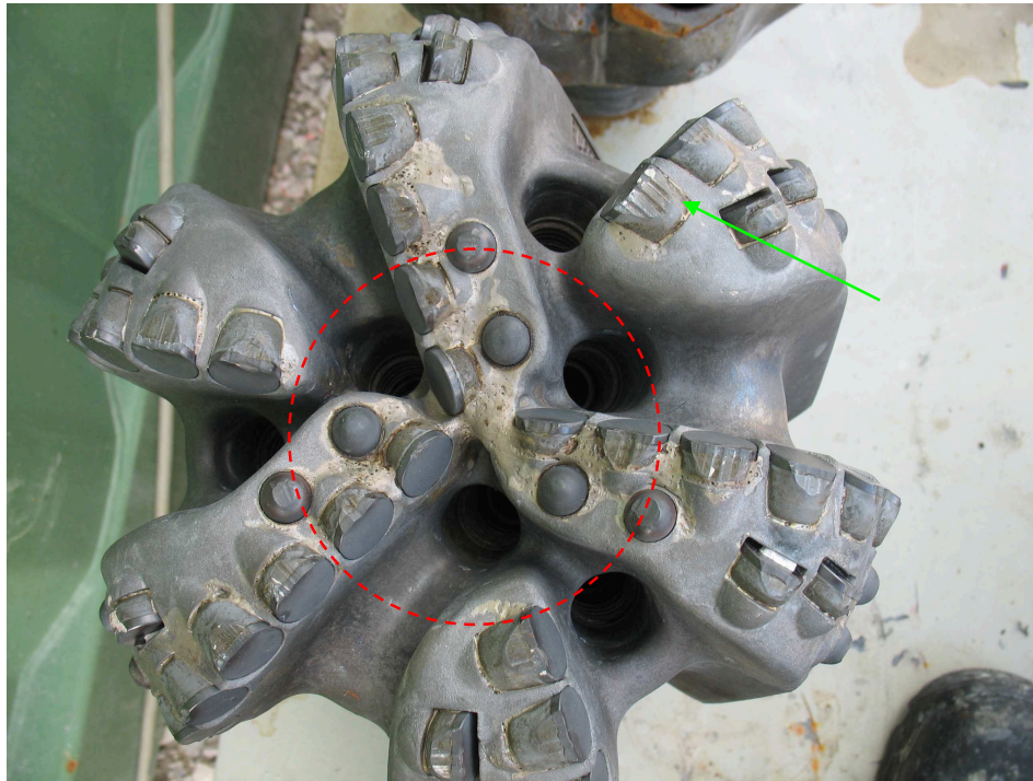
Figure 8.10 – OKSP-001 run #8: PDC with dome-topped inserts preventing a ring out, high wear though at outer cutters
