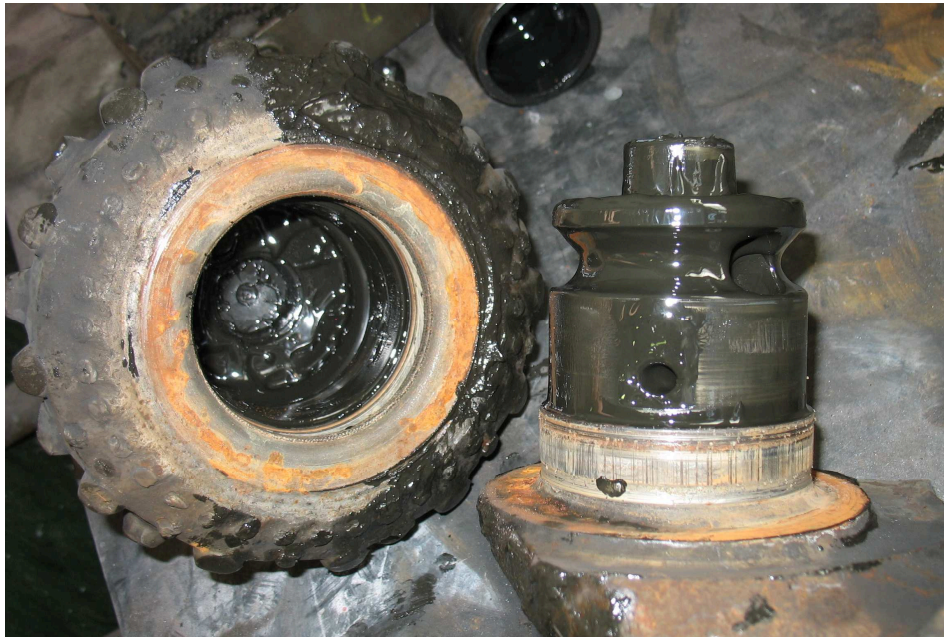
Figure 5.3 – Dismounted cone – bearing and leg with remaining lubricant
