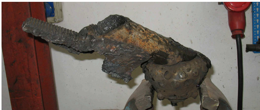
Figure 5.1 – Disassembled leg after arc welding
