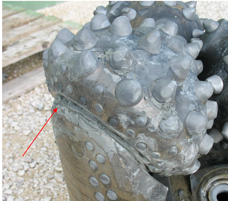
Figure 8.9 – OKSP-001 run #4: roller cone bit with seal breakage and mud intrusion
