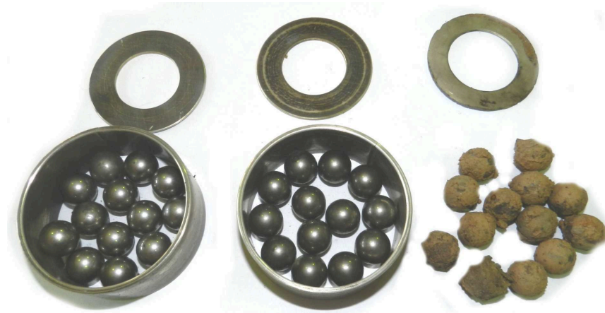
Figure 5.5 – Internal bearing components (#3 components show strong mud intrusion)
