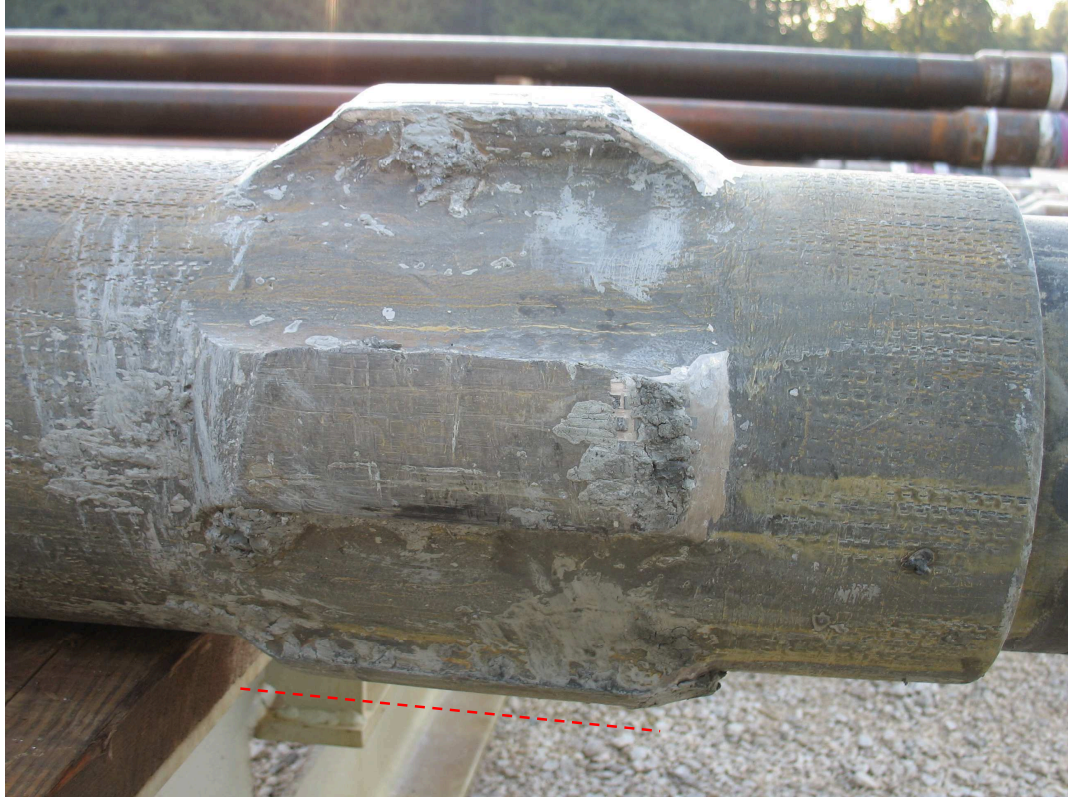
Figure 8.7 – OKSP-001 run #3: bearing sub with extensive wear on low side
