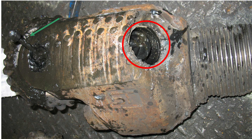
Figure 5.2 – Dismantled pin (green) and reservoir section (red)
