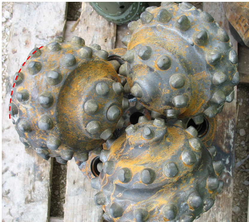
Figure 8.8 – OKSP-001 run #3: roller cone bit with minor signs of wear
