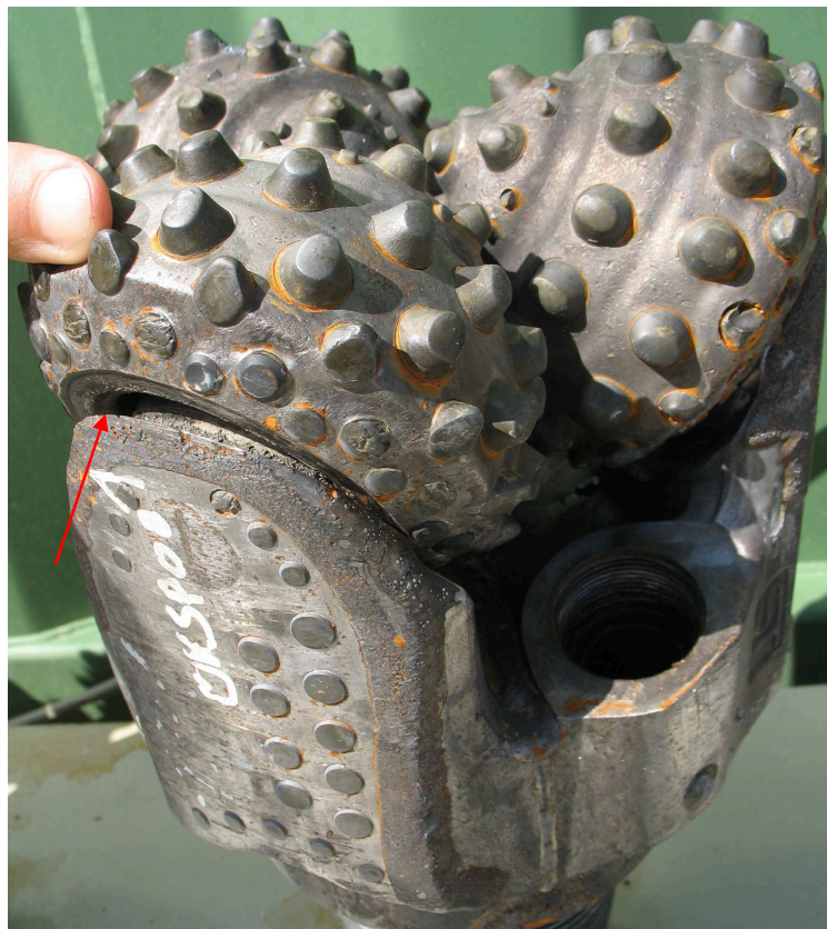
Figure 8.11 – OKSP-001 run #9: loose cone at TCI after 46.5 hours
