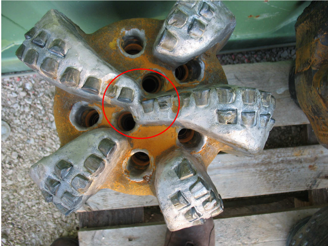
Figure 8.3 – OKSP-001 run #1: PDC with a ring out and worn teeth
