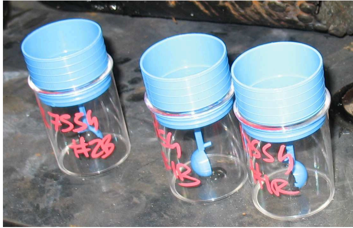
Figure 5.4 – Collected grease samples, ready for grease – water analysis
