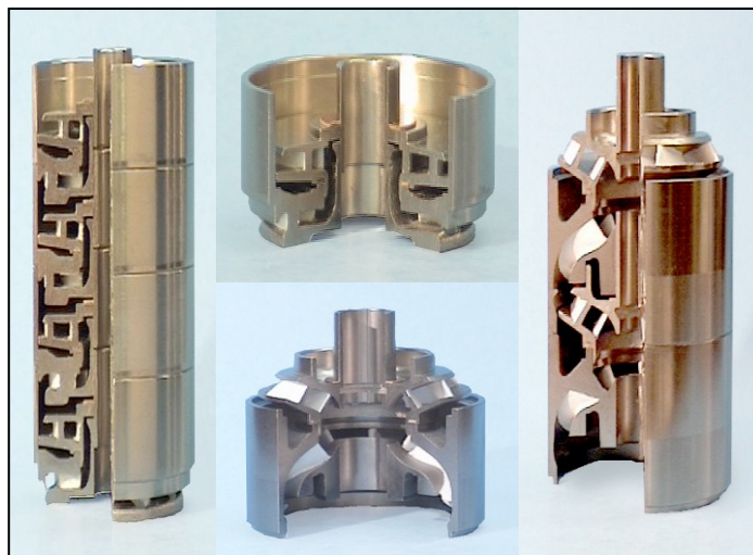
Figure 7 Type of flows (radial and mixed flow) (7)
