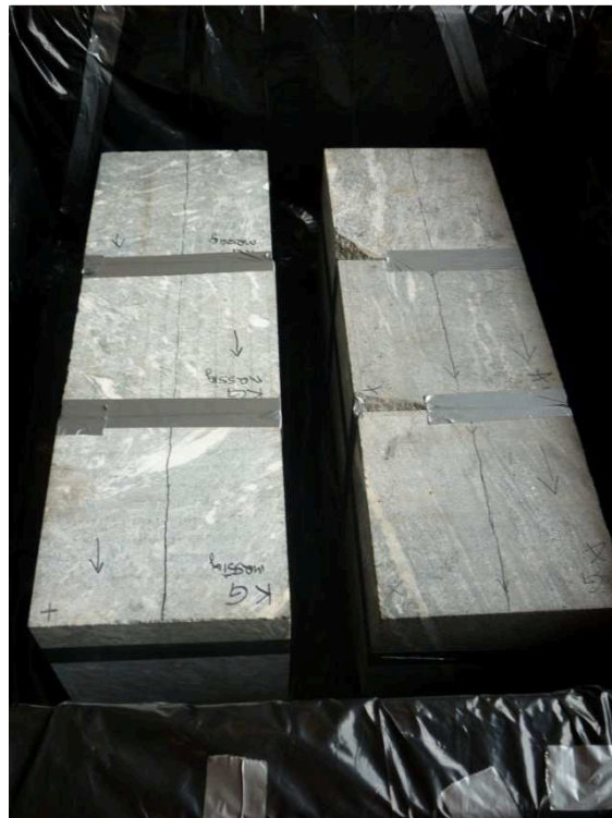
Figure 15: Rock cubes placed in the metal box lined with plastic sheeting
