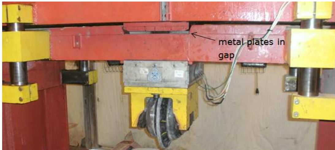
Figure 9: Cutter penetration spacers in place
