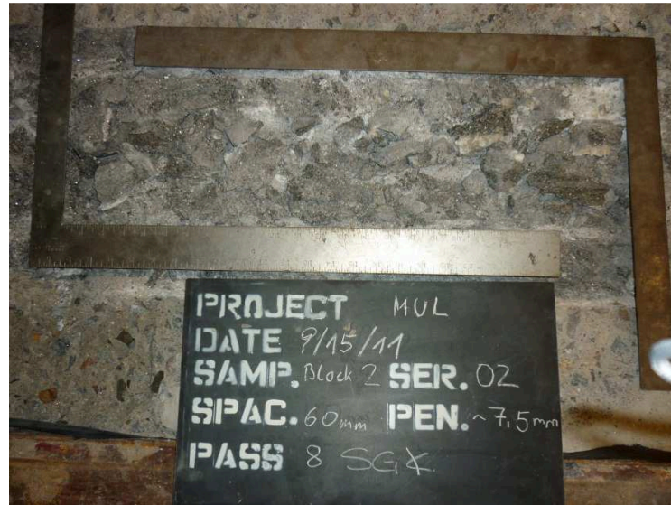
Figure 21: Area between squares for schistose gneiss, series MUL02, pass 08, spacing 60 mm and penetration 7.6 mm
