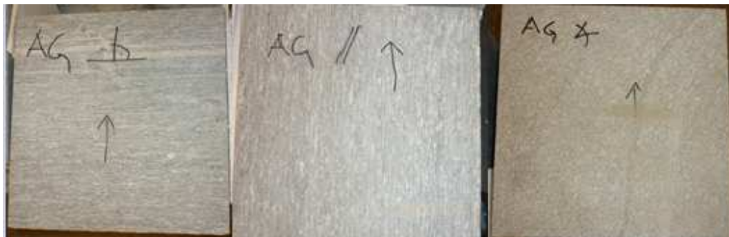
Figure 12: Rock cubes of augen gneiss with perpendicular, parallel and oblique foliation direction
