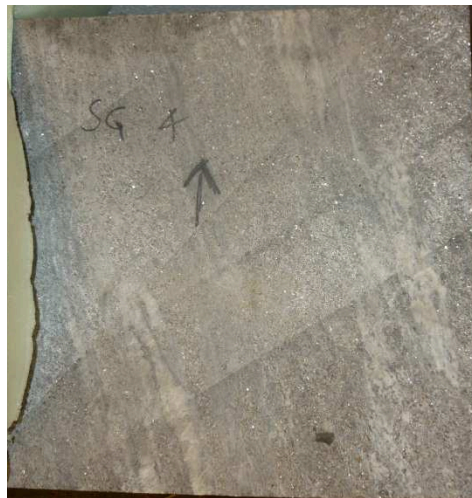
Figure 13: Rock cube of schistose gneiss with oblique foliation direction
