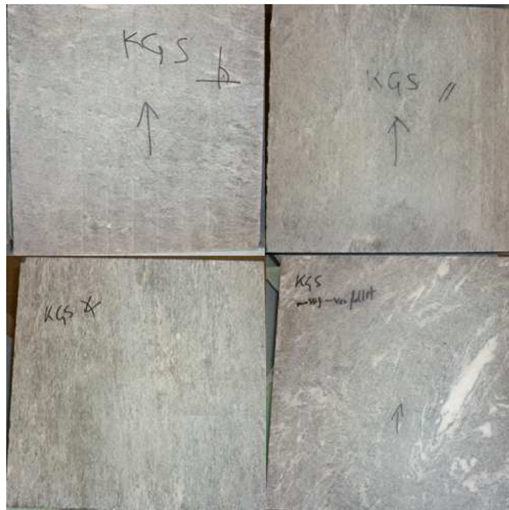
Figure 11: Rock cubes of calcareous mica schist with perpendicular, parallel, oblique and massive foliation direction
