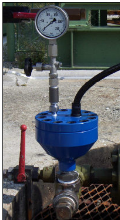
Figure 23: Measurement devise of MURAG system. (Sam, Kästenbauer, Burgstaller, & Chevelcha, 2012, Page 8)
