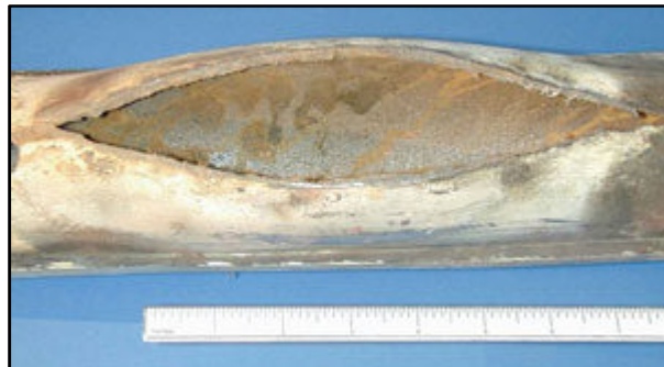
Figure 18: Example of hydrogen blistering. (Daniels, 2012)
