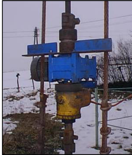
Figure 26: ECRR system installation.
