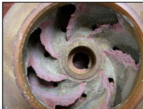
Figure 19: Example of erosion. (Pair O Docs, 2012)
