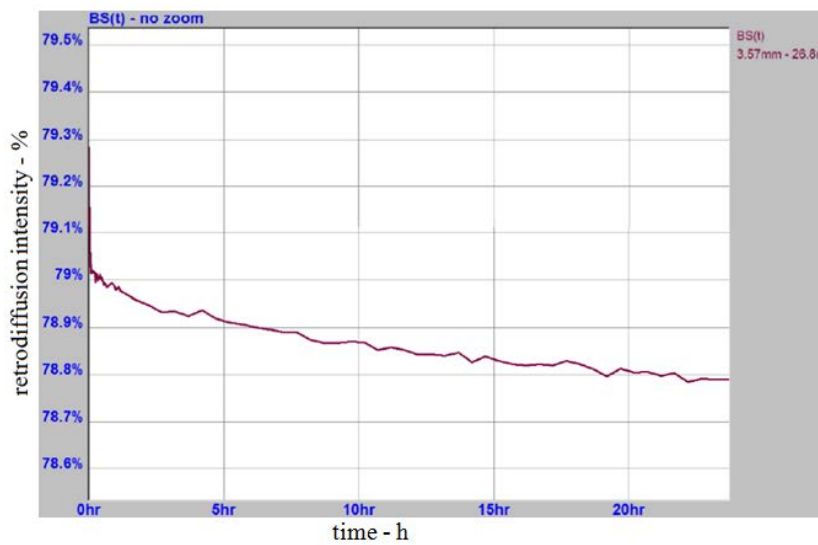
Figure 4.5: Evolution of the backscattering signal with time at a suspension of 40 vol.% Durcal 5 and the glucose-water mixture.
