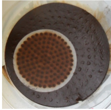
Figure 9-6: Filter cake of Fe-Mn residue
