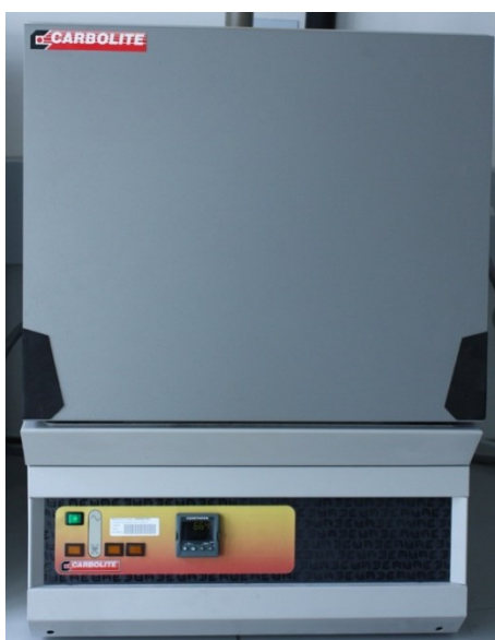
Figure 8-4: Carbolite incineration furnace AAF 12 18 1200 °C
