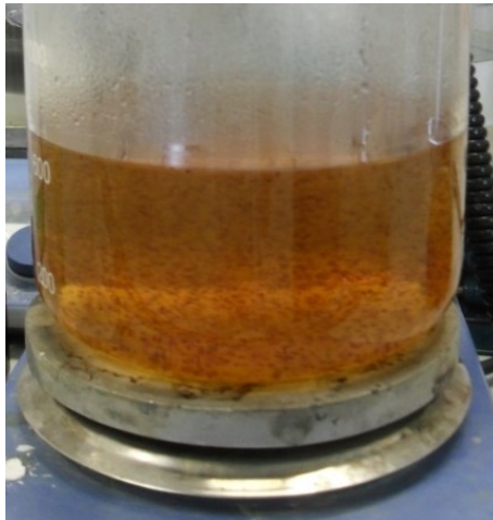
Figure 9-5: Solution with partly reacted \text{KMnO}_4 (solution with dispersed Fe-Mn precipitate)
