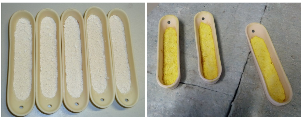
Figure 8-5: Left: Sample material before treatment (white); Right: Sample material directly after the treatment at 900 °C (yellow ZnO)
