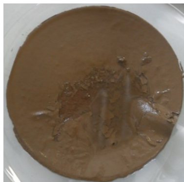
Figure 9-4: Filter cake of lead residue
