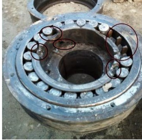
Figure 3-23. Consequence of washout wiper seal on the crosshead bearing (A.Samuelson, 2020)
