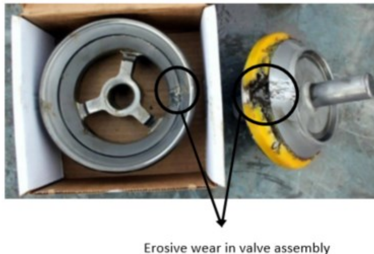
Figure 3-21. Valve and seat failure due to high operating pressure and abrasive drilling fluid (V.Ulmanu, 2016)
