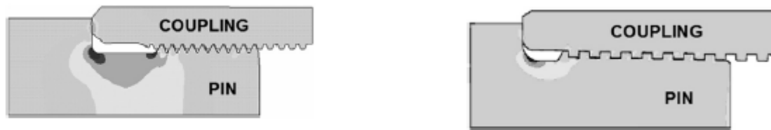
Figure 2.9: Comparison of the geometry and stress distribution in the API connection (left) versus a premium Tenaris connection (right) [14, p. 27]
