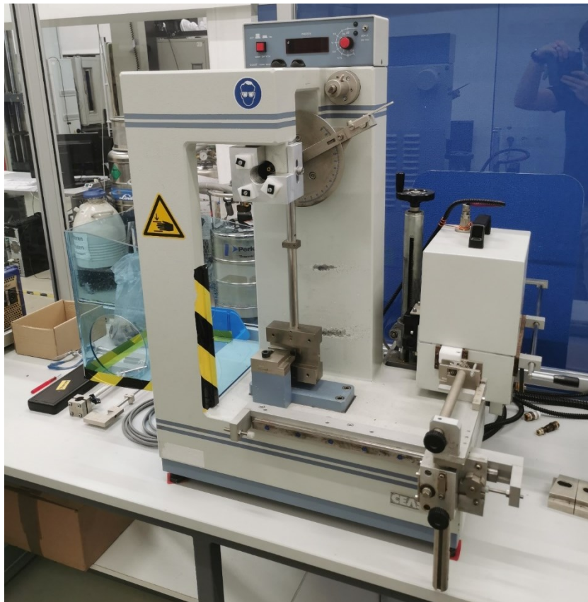
Figure 3.18: Charpy impact test setup.
