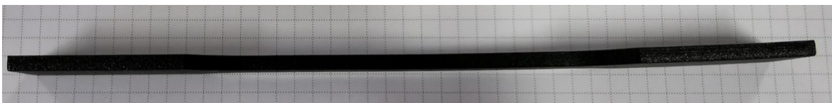
Figure 3.14: Warped specimens after delivery of a TPP.
