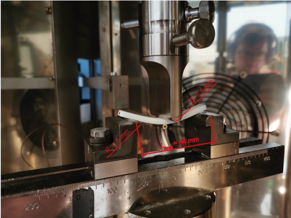
Figure 3.20: 3PB setup while testing.
