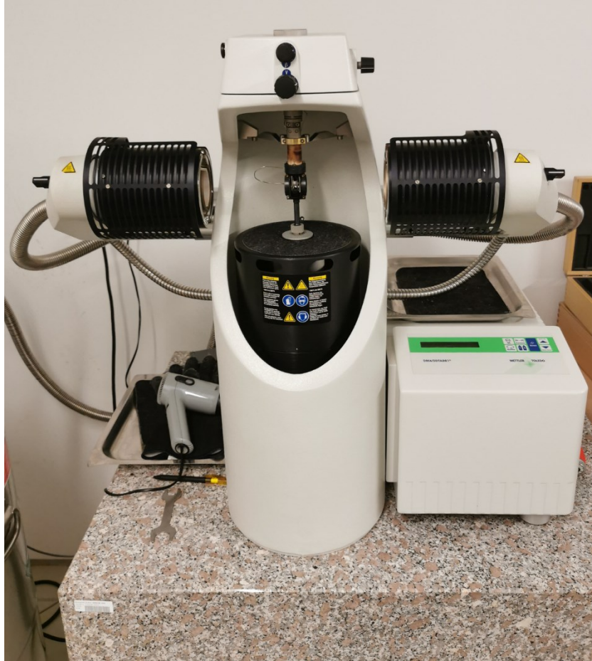
Figure 3.17: 12 N DMA “DMA/SDTA861 e ” from Mettler Toledo, USA.
