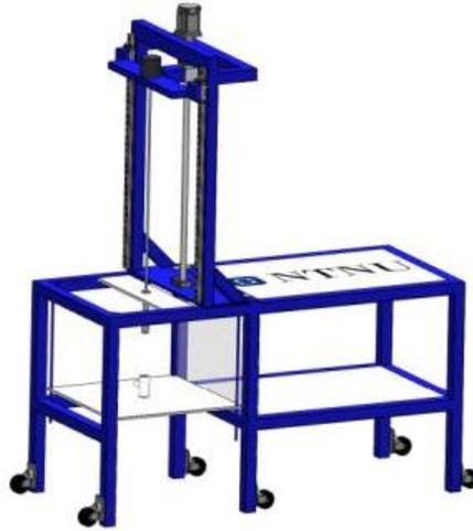
Figure 2.13 – NTNU laboratory drilling rig (Lescoeur et al., 2017)
