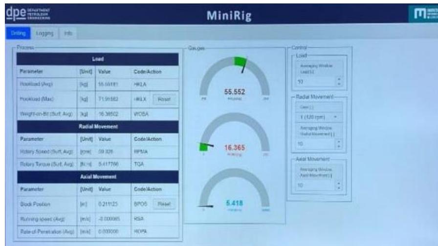
Figure 3.5 – Page with drilling parameters
