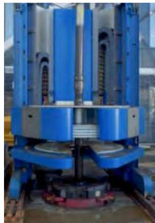
*Figure 2.7 – Robotic Roughneck (Raunholt et al., 2021)*
