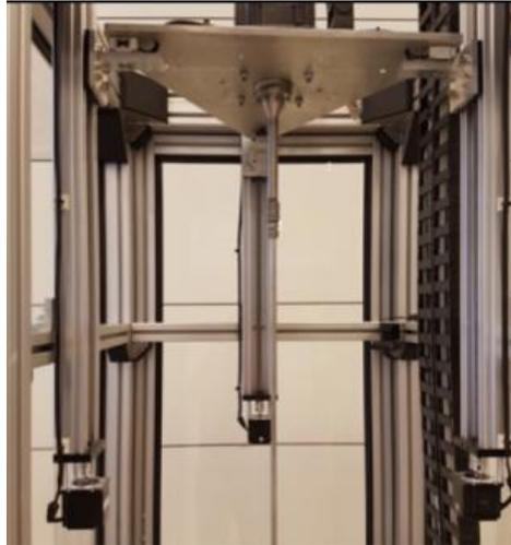
Figure 2.15 – Hoisting system with stepper motors (Løken and Løkkevik, 2019)
