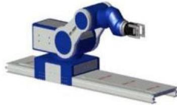
*Figure 2.5 – Drill Floor Robot (Cappuccio et al., 2019)*
