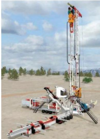
*Figure 2.9 – Automated tripping operations system (Mul et al., 2020)*
