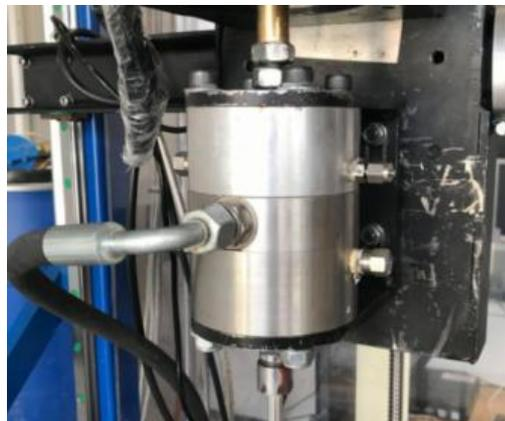
Figure 2.20 – Swivel and diverter (Alvarez et al., 2022)
