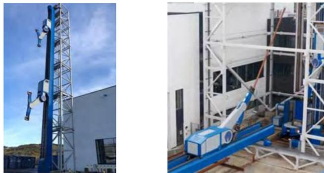
*Figure 2.6 – Robotic Pipe Handler and Pipe Deck Handler (Raunholt et al., 2021)*
