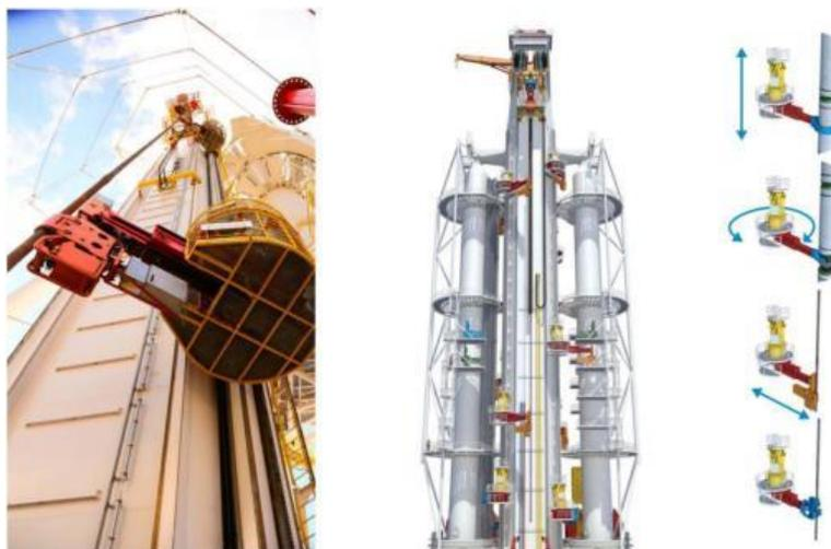
Figure 2.12 – Manipulators of drill stands (Roodenburg et al., 2017)
