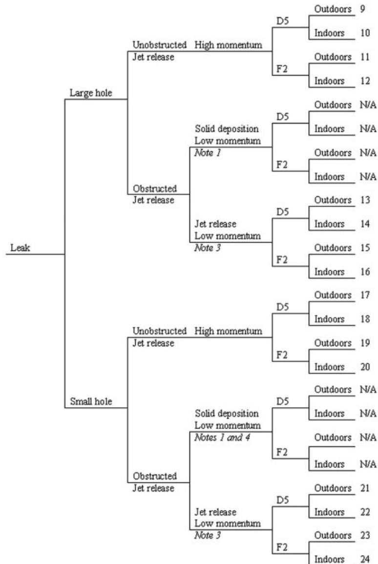
Figure 15 – Holes in the pipeline event tree (McGillivray, A. et al., 2014)
