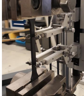
Figure 18: Makro positioning on multipurpose specimen, tensile test setup.
