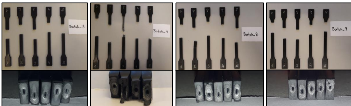
Figure 32: Blowholes of B3, B4, B8 and B9.
