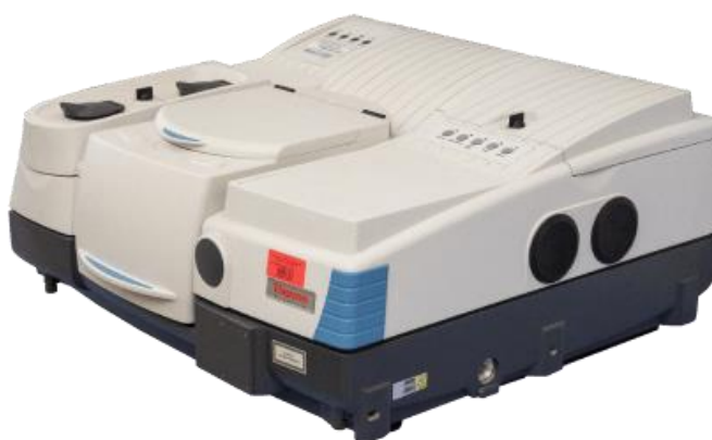
Figure 8. Nicolet 6700 FT-IR spectrometer
