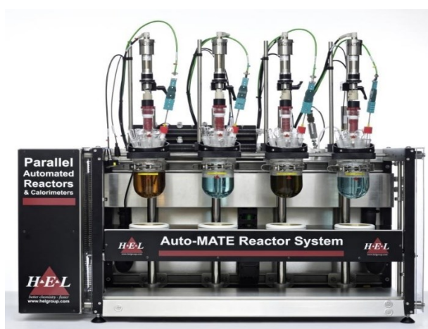
Figure 4: Automatic chemical process control system HEL Auto-MATE Reactor System
