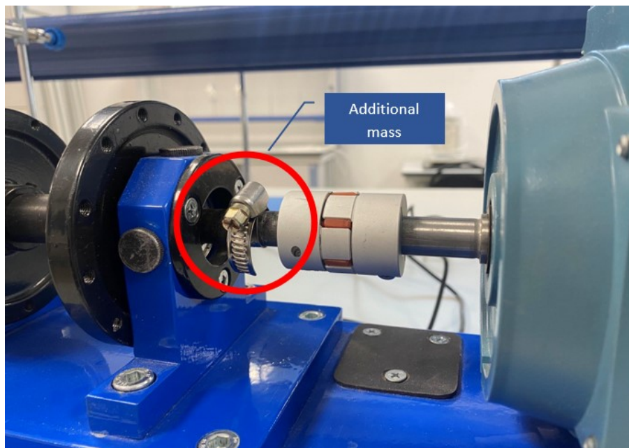
Figure 3.20 - Adding additional mass to the rotor to create rotor imbalance
