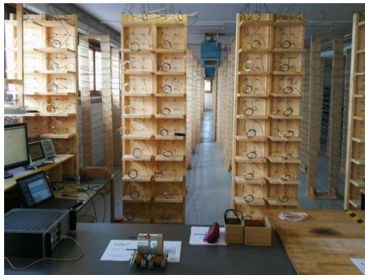
Figure 28 - 8 km conduit test bench
