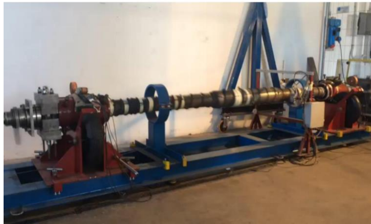
Figure 25 - Test bench for fatigue failure of joints
