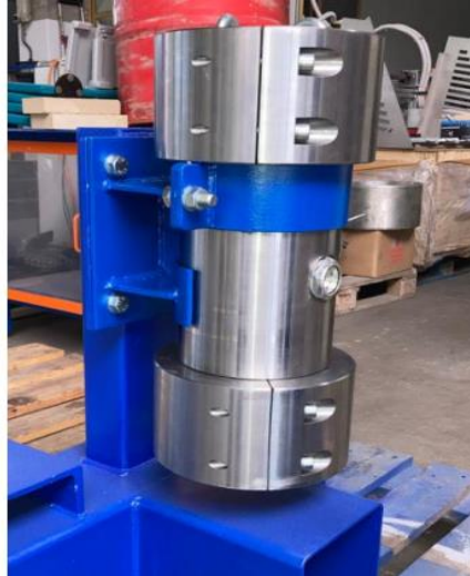
Figure 27 - High pressure double-shoulder main sealing test bench
