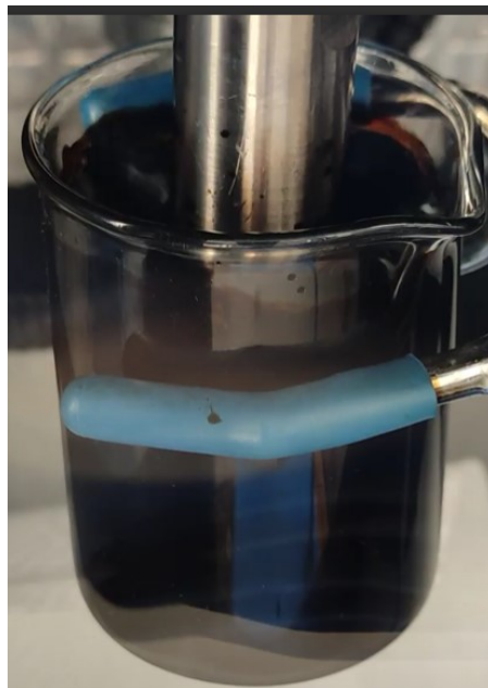
Figure 4.12 – Boiling like characteristic of surface
