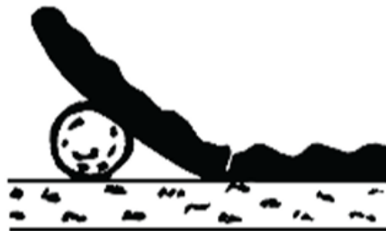
Separation piece of film from the surface at pulsation bul
