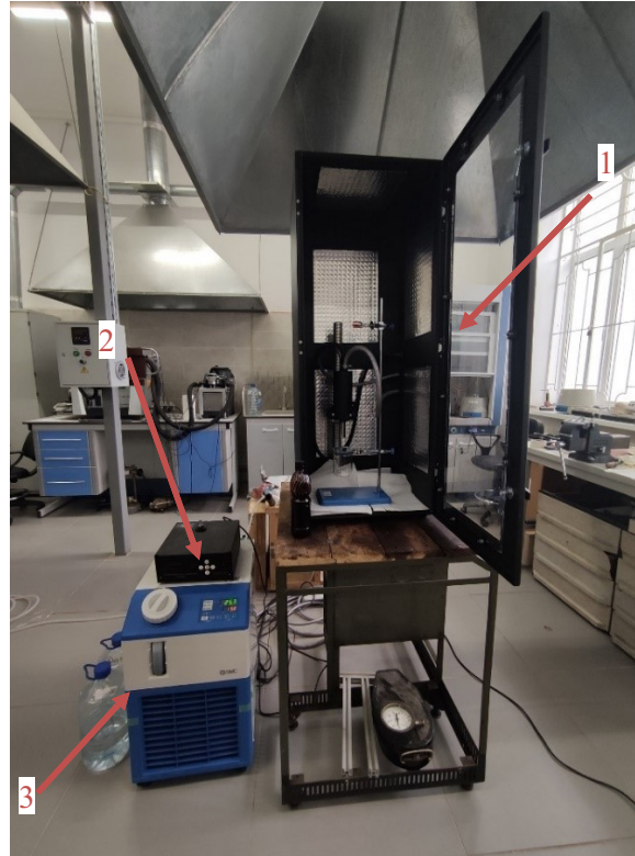
Figure 3.10 – Ultrasonic treatment unit, 1 – cabinet, 2 – control device, 3 – thermostat
