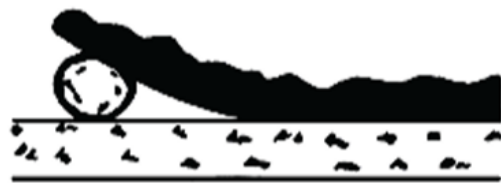
Formation of a bubble at the surface under a layer
