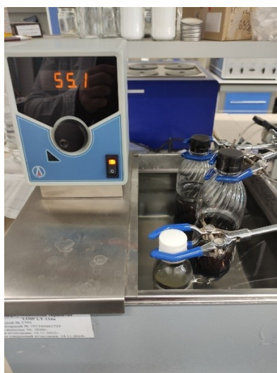
Figure 4.16 – Oil and additives in thermostat
