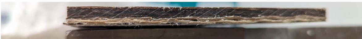
Figure 27: Ply displacement of layers in vitrimer-based specimen repair trial due to excessive load.
