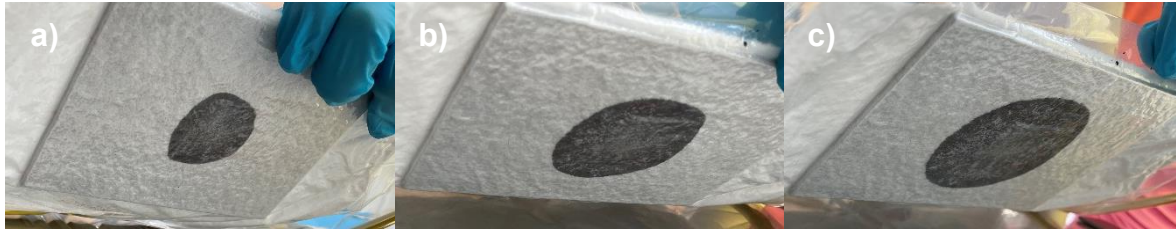
Figure 14: Injection repair process. a) After 1 minute. b) After 5 minutes. c) After 10 minutes
