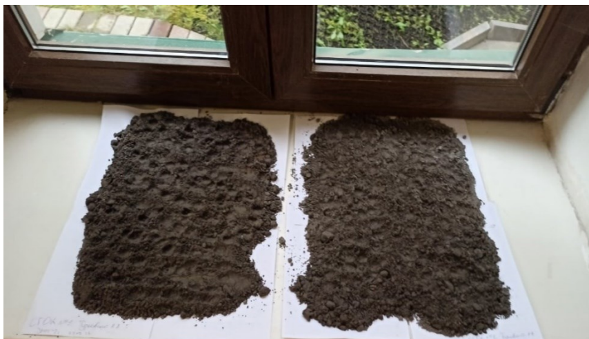
Figure 4: Figure 4 - Drying of Iron ore tailings
