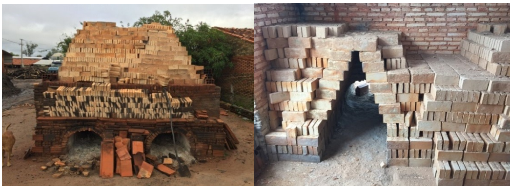
Figure 28: Basic Caipira from the outside and inside
