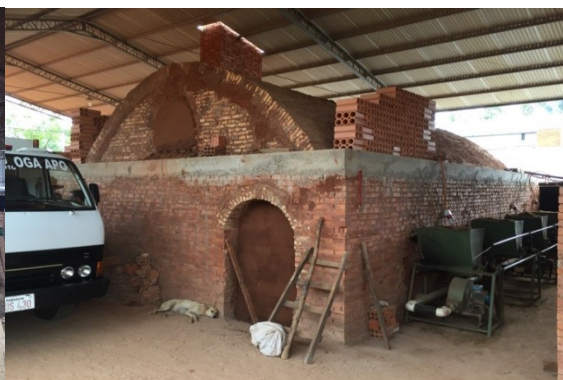
Figure 27: Albert kiln fired with sawdust
