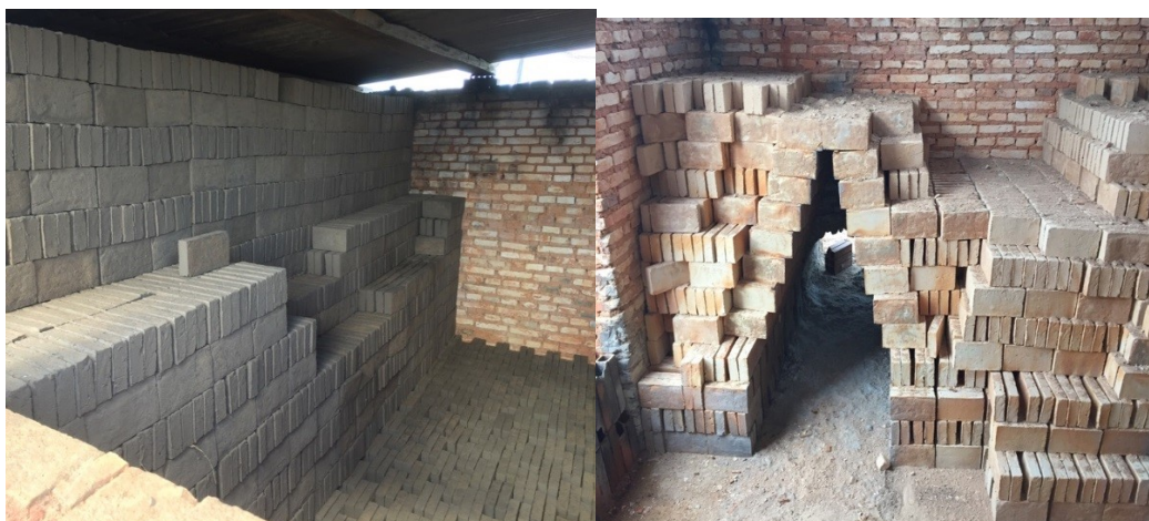
Figure 60: stacking of ladrillo comunes in Capira kiln
