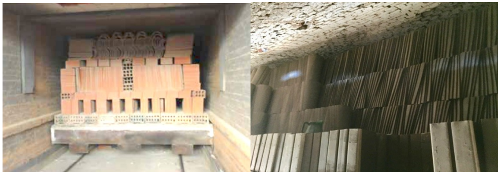
Figure 42: Tunnel and Albert kiln filled with roof tiles
