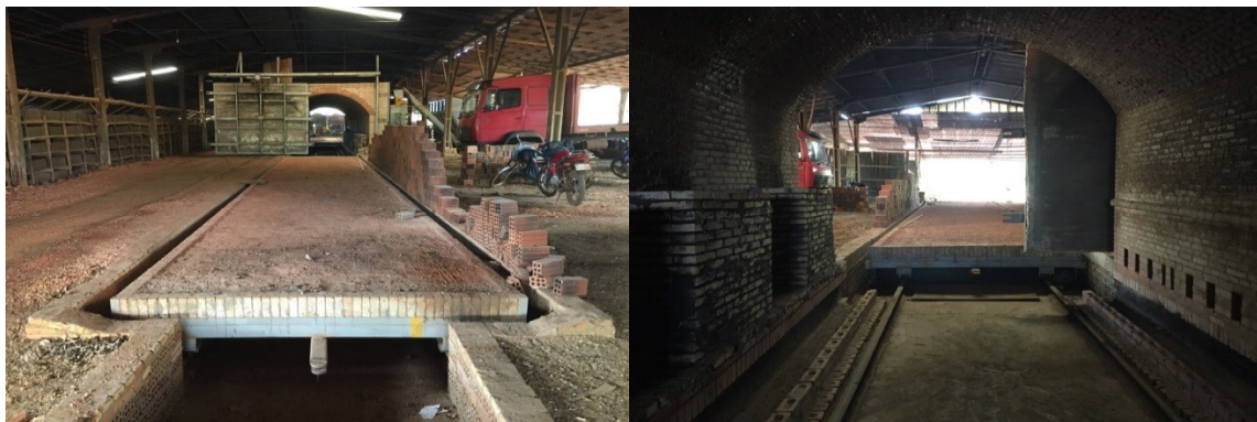
Figure 25: Wagon kiln near Ciudad del Este
