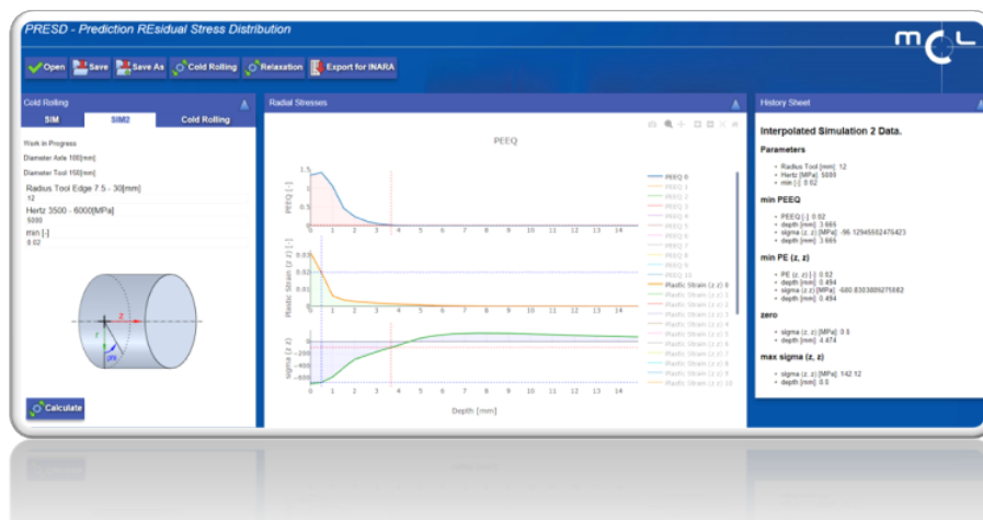
Figure 3.17: GUI of the PRES D software tool. Left: definition of input parameters. Center: stress and strain distributions. Right: input and result history.
