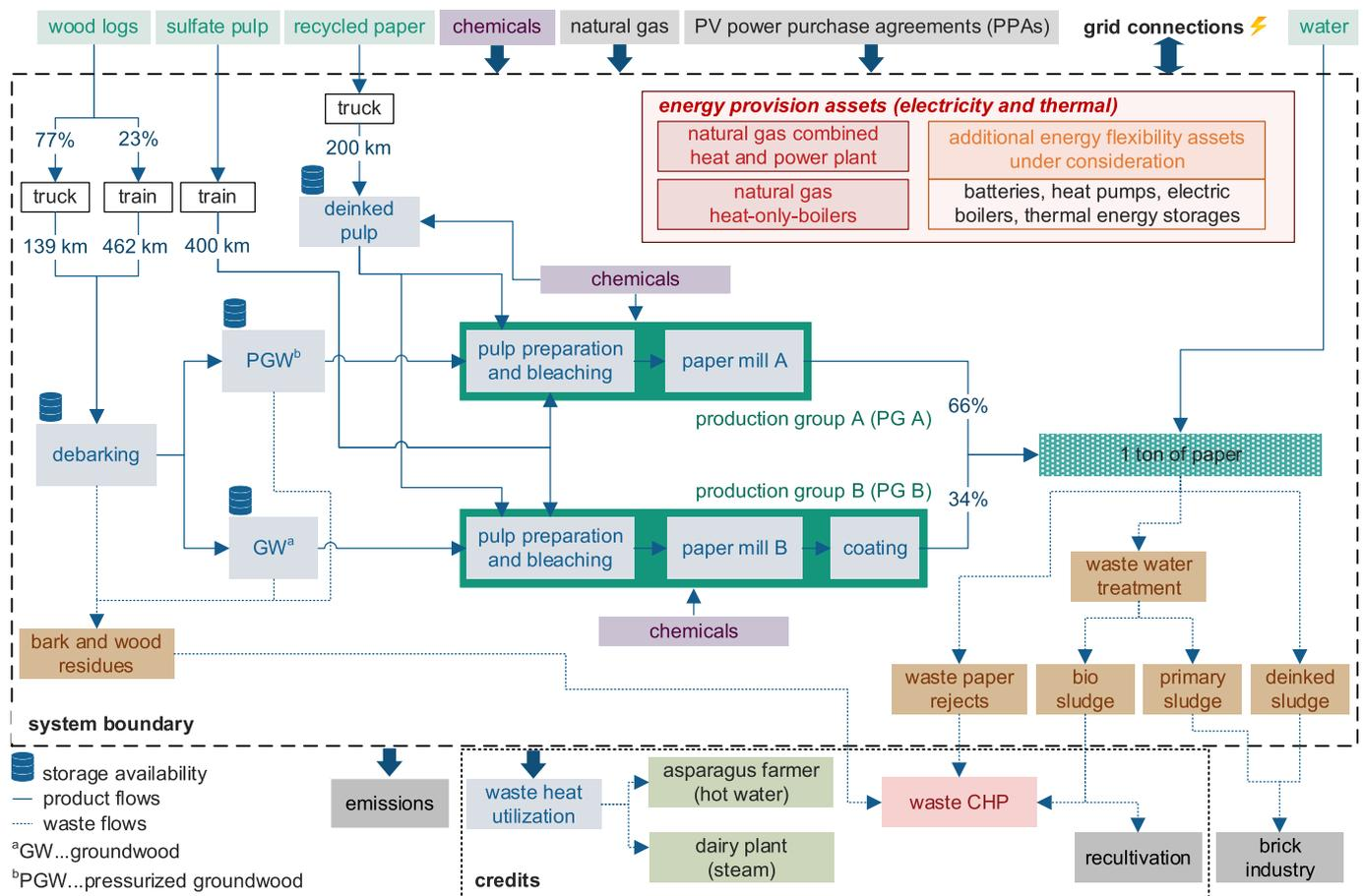
Fig. 4. System boundary of exemplarily analyzed system in the pulp and paper industry.
