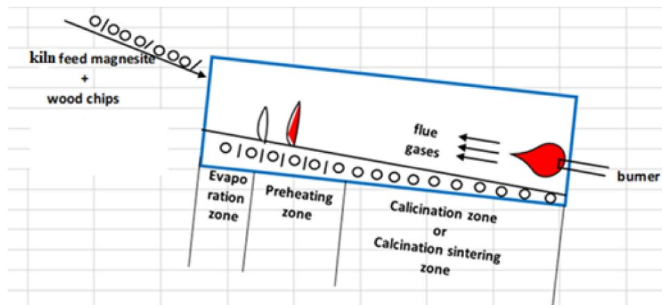
1. Evaporation zone (Temp~400–500 °C) : The moisture is evaporated
