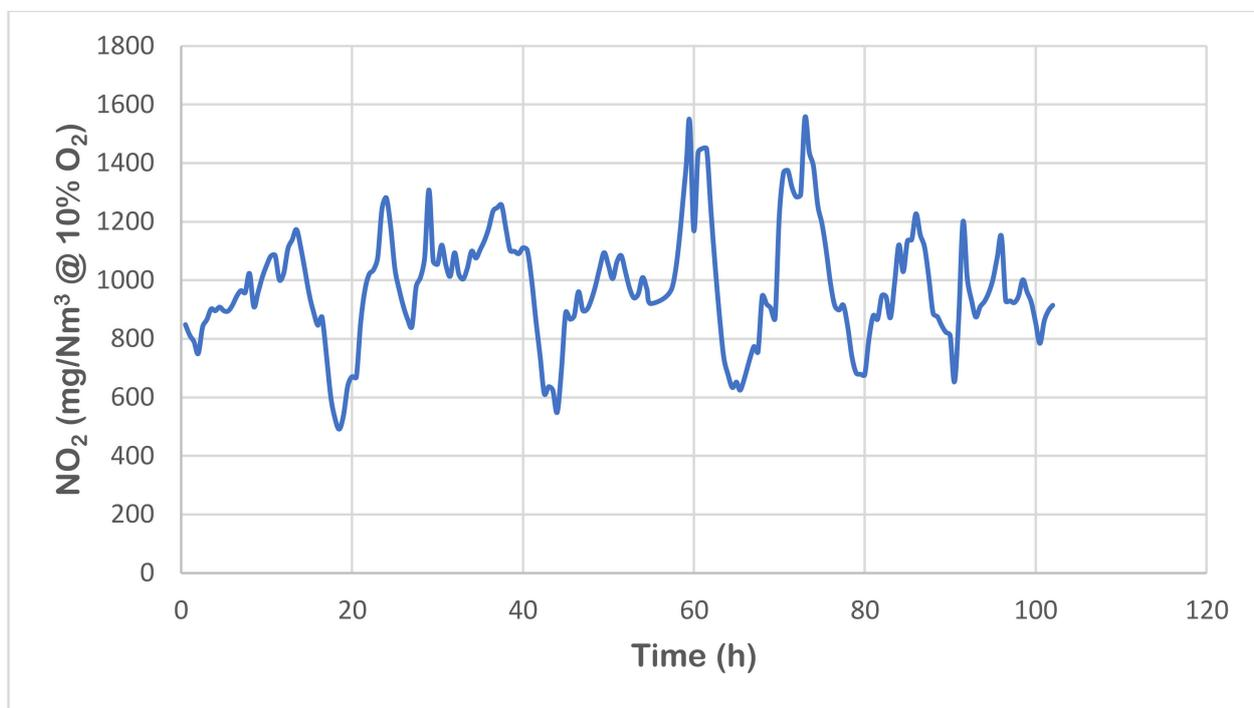
**Figure 6.** NO<sub>2</sub> pollutant concentration in flue gases during 100% pet-coke trial. NO<sub>x</sub> trial average is 980 mg/Nm<sup>3</sup> at 10% O<sub>2</sub>.
