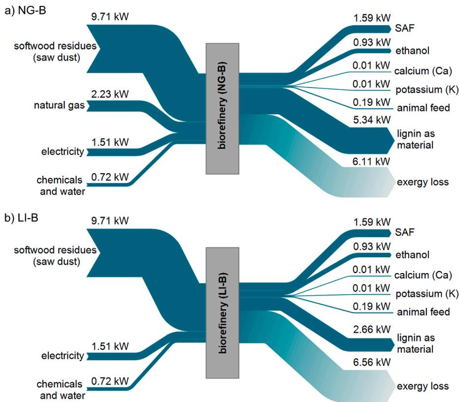
Fig. 8. Exergy flows of biorefinery to produce 1 t<sub>SAF</sub> for scenario a) NG-B and b) LI-B.
