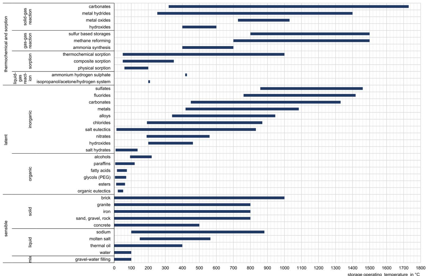
Fig. 3. Theoretical storage operating temperatures of thermal energy storage types.
