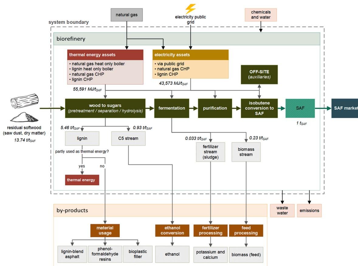
Fig. 3. Biorefinery concept and system boundary to produce SAF.
