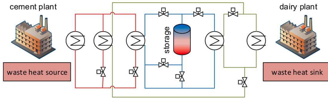
Fig. 2. Flow sheet showing waste heat recovery (red), storage (blue), and transportation (green), based on [40].
