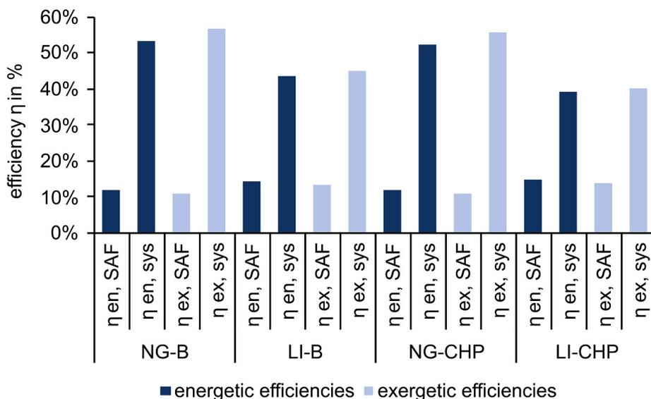
Fig. 7. Energetic and exergetic efficiencies of biorefinery.
