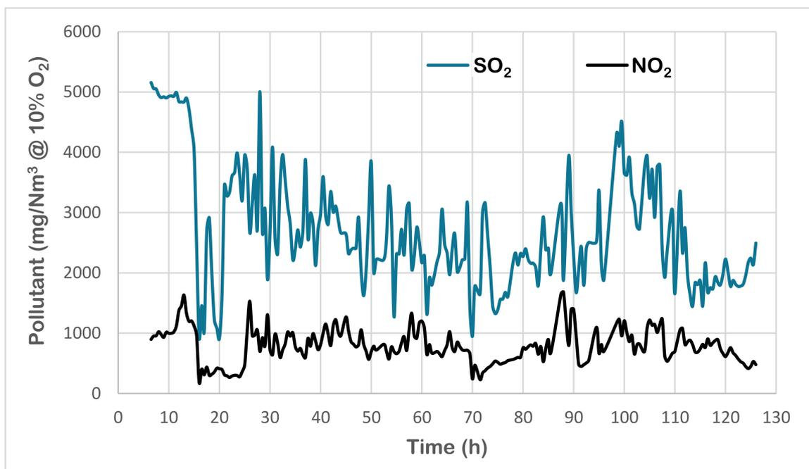
**Figure 7.** SO<sub>2</sub> and NO<sub>2</sub> concentration of the flue gases at kiln exit during the 5-day trial (February 2022).
