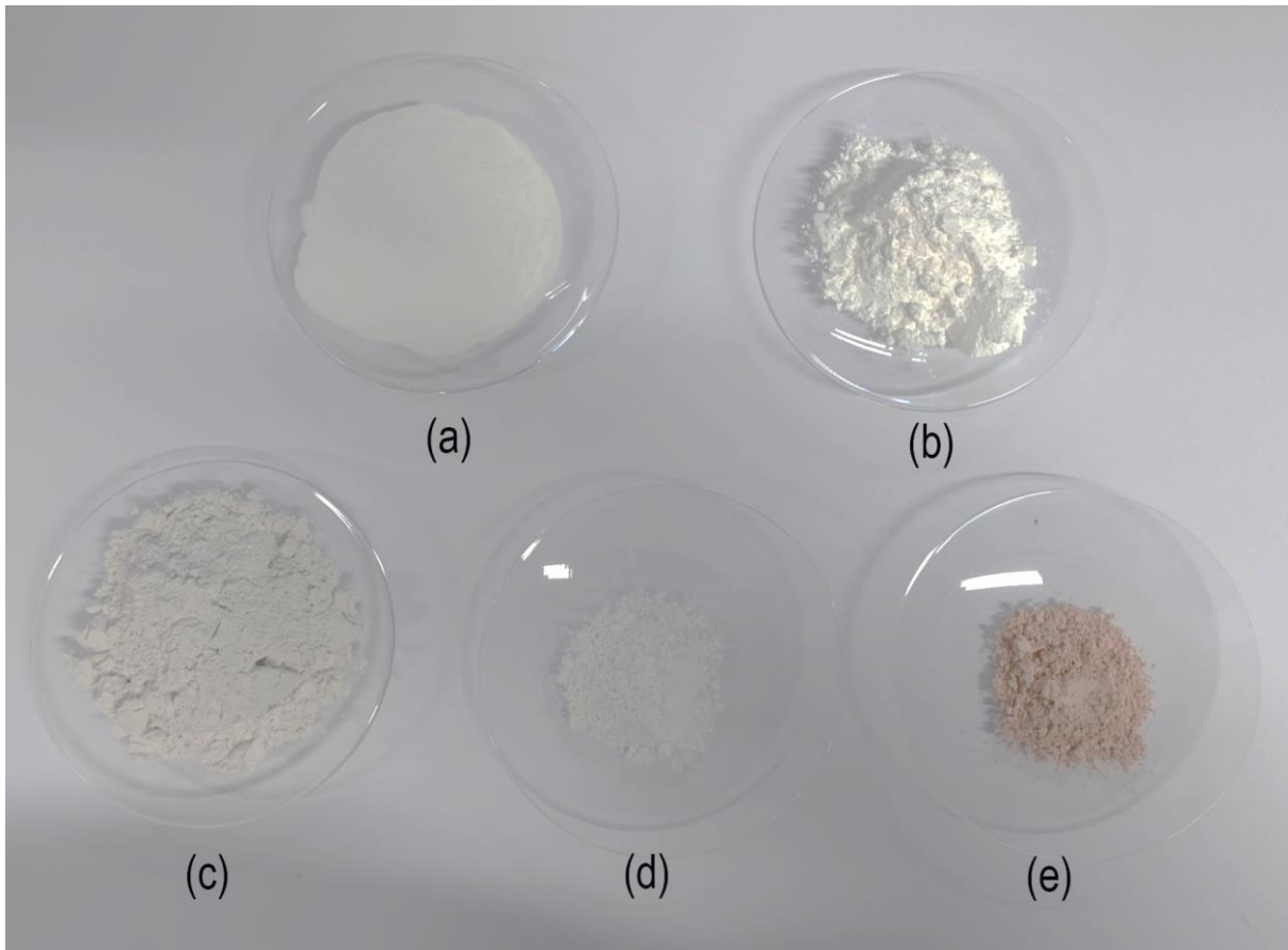
Figure 7. Raw oxide materials used in the investigations, (a) calcium oxide, \text{CaO} ; (b) magnesium oxide, \text{MgO} ; (c) silicon dioxide, \text{SiO}_2 ; (d) aluminum oxide, \text{Al}_2\text{O}_3 ; and (e) cerium dioxide, \text{CeO}_2
