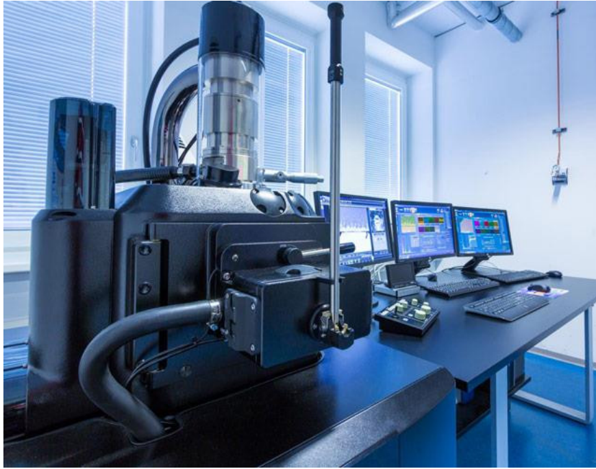
Figure 10. Scanning Electron Microscope (SEM) equipped with an energy dispersive X-ray (EDS) detector used in the investigation
