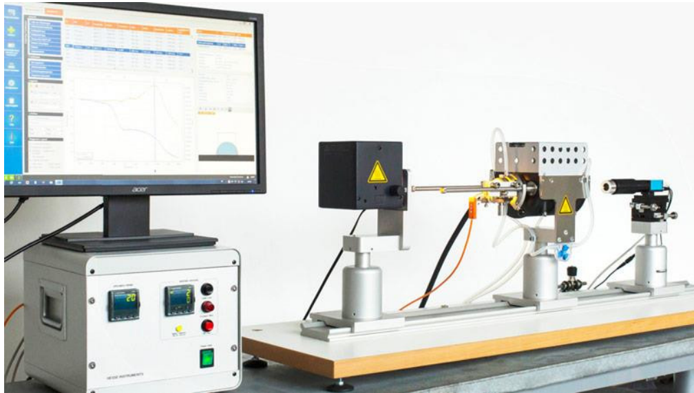
Figure 9. Hot stage microscope used to observe melting behavior of slag samples
