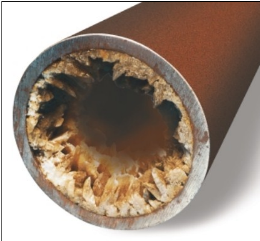
Figure 2: Scaling in Production Tubing [22, p. 1]
