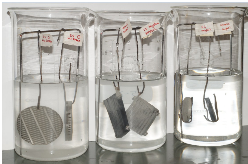
Figure 16: Experimental Setup for Part 2 of Scaling Behaviour Test- Scale Removal
