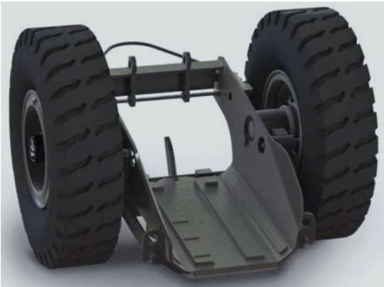
Figure 03: Base frame and stub-axels [1].
