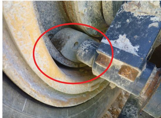
Figure 04: Automatic safety brakes.
