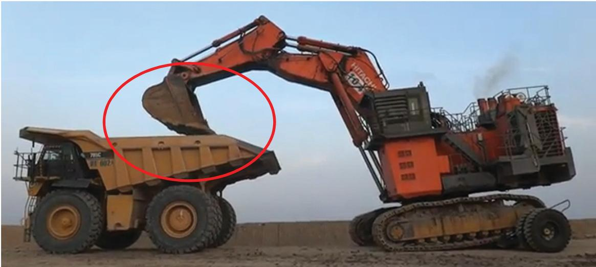
Figure 07: Dumper driving backwards under the boom of the excavator [4].
