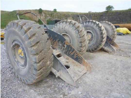
Figure 32: Slepner E90-750 from Hope Works.
