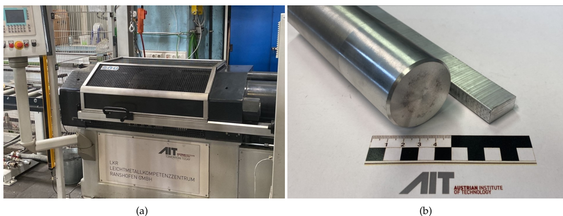
Figure 1.11.: Pictures of (a) the used 1.5 MN extrusion press (NEHP 1500.01, Müller Engineering), (b) cast feedstock and extruded square profile.
