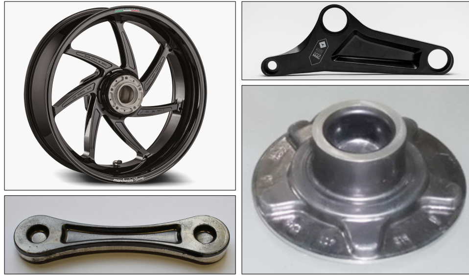
Figure 2.1.: Various Mg forged parts, showing (u.l.) a motorbike rim produced by Brembo S.p.A. under Marchesini trademark, (u.r.) a bike suspension link made by ALLITE® Inc., (b.l.) laboratory scale piston rod forged by Light Metals Technologies Ranshofen and (b.r.) a wheel hub produced by Institut für Metallformung, University Freiberg. Reproduced with the kind permission of: Brembo S.p.A., ALLITE® Inc., Light Metals Technologies Ranshofen and TU Bergakademie Freiberg.
