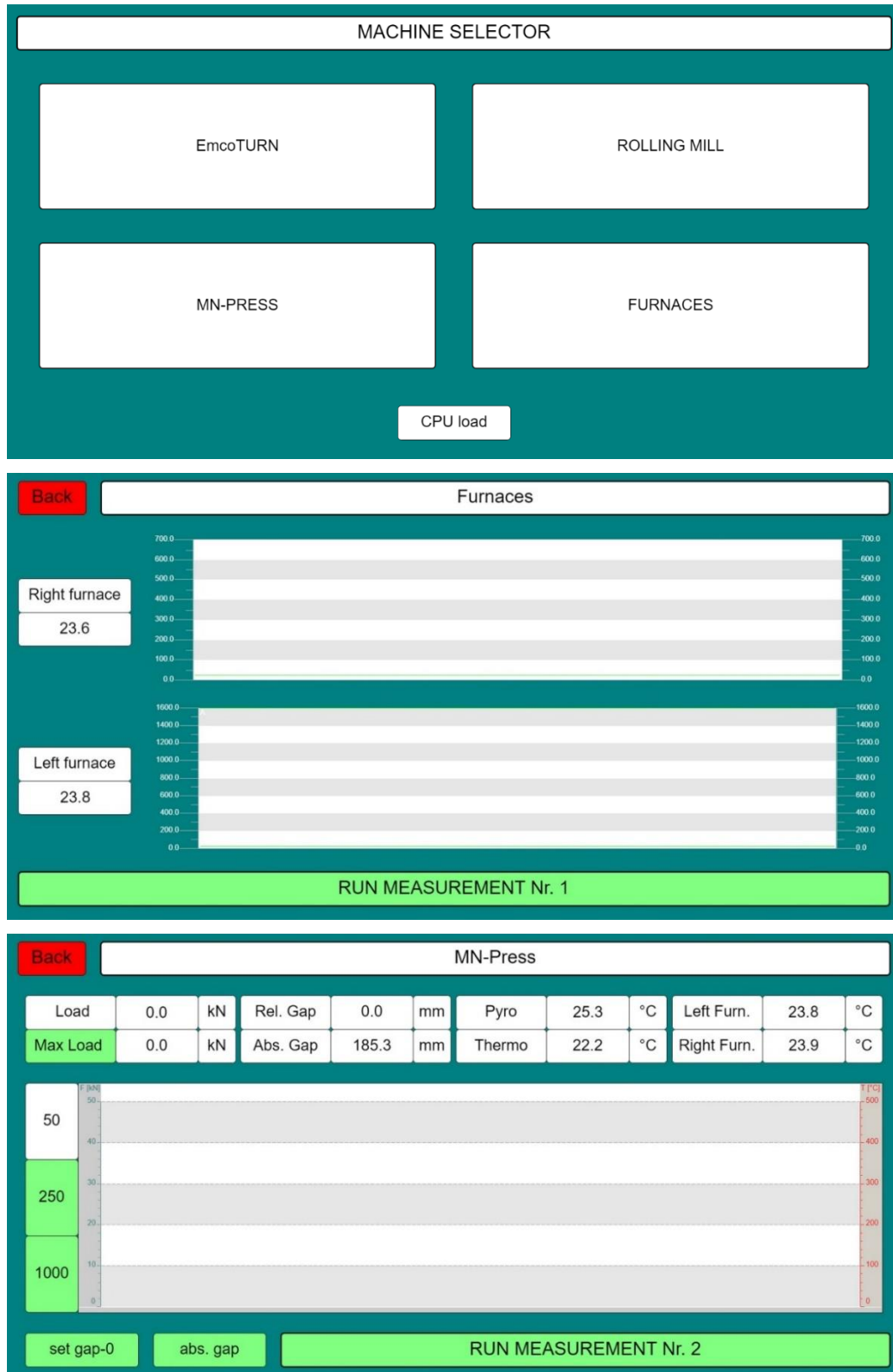
Fig. 11. Superordinate WAGO GUI (top), GUI of both furnaces (middle), and GUI of the hydraulic press (bottom) [124]
