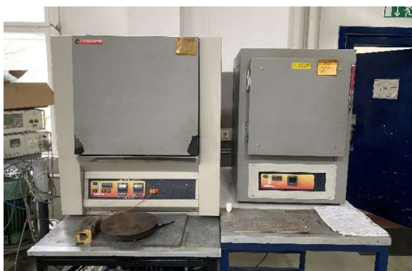
Fig. 5 Furnace 1 (right) capable of 600°C and furnace 2 (left) capable of 1400°C
