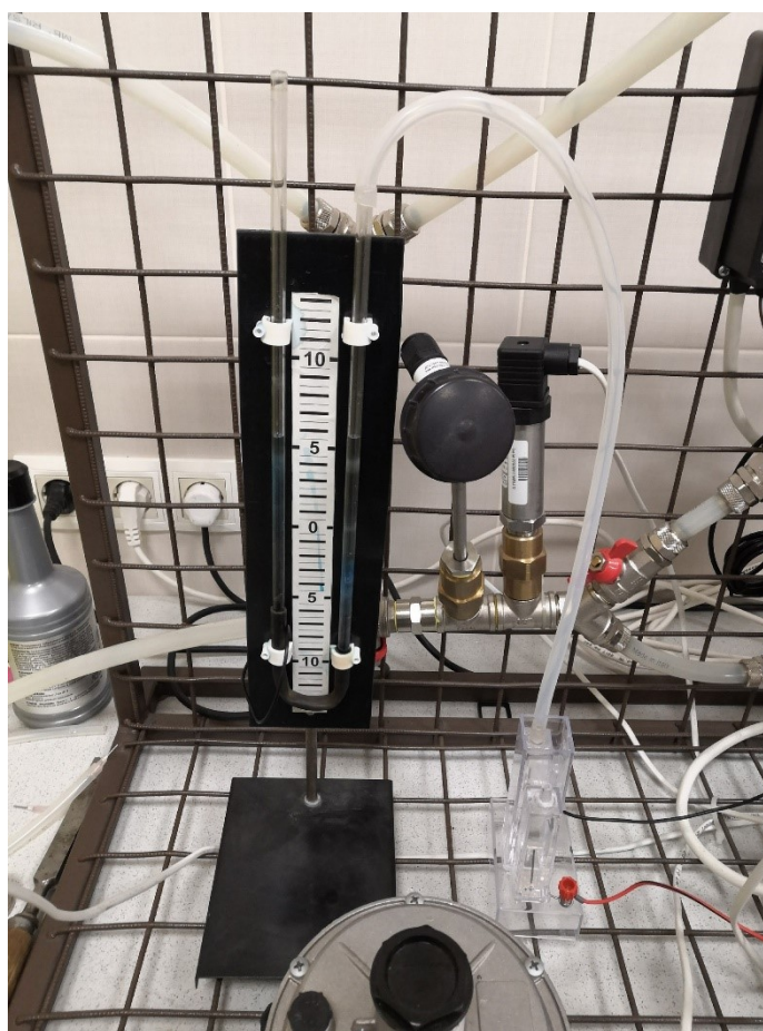
Figure 17: Manometer The height of the displaced liquid column indicates the hydrogen pressure, the volume of the manometer is known. According to the equation of state of the gas, we determine the masses of hydrogen and the volume under normal conditions.
