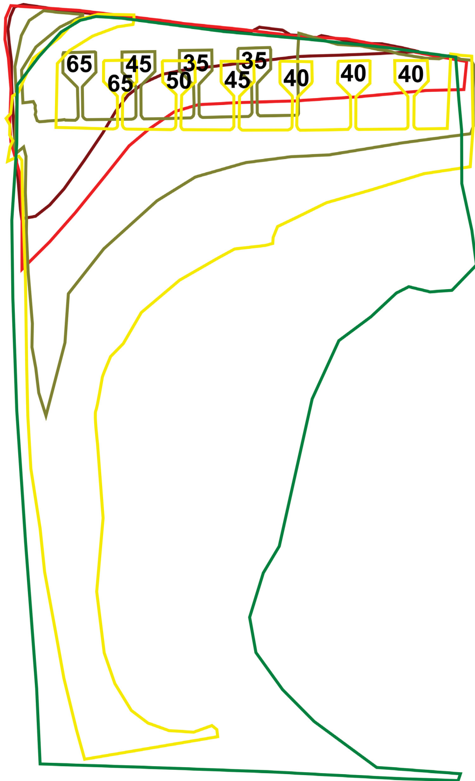
Figure 8.1: Outlines of the aligned thin sections of the sample HST B with the reconstructed average sampling depth (in \mu\text{m} ) noted in the head of tensile specimens.
