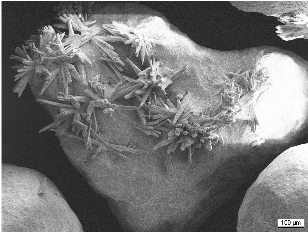
Figure 53 - Crystallization of calcium carbonate on the surface of ceramic grain after static test.
