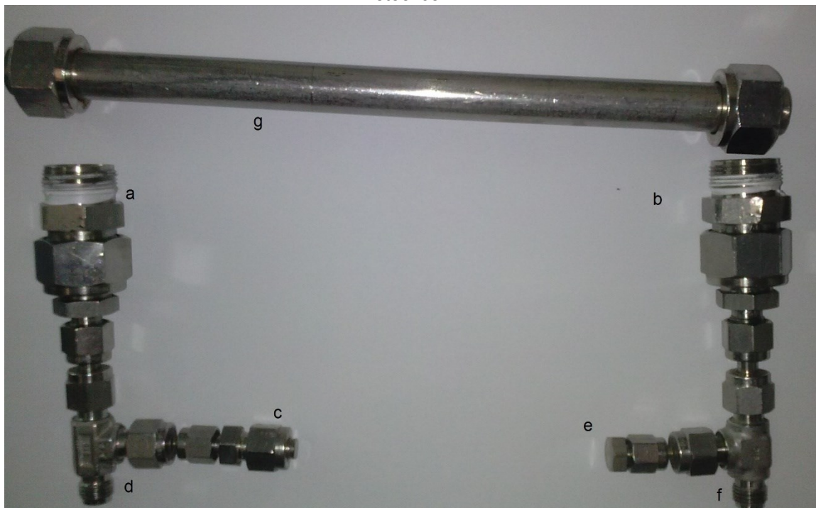
Figure 33 - second steel cell with 1.18 cm diameter. a,b)inlet or outlet connection to cell with sieve d,f)inlet or outlet connection from pump c,e)connection to pressure transducer g)the cell
