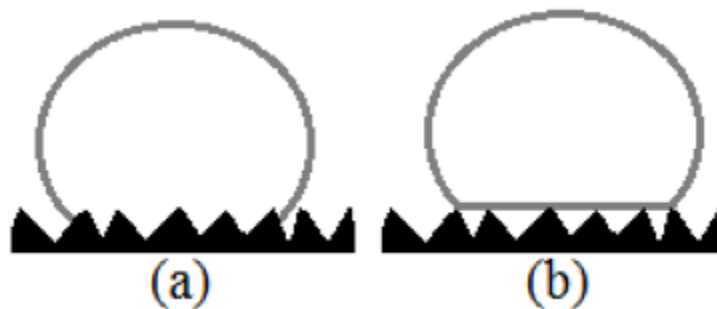
Figure 19 - The different wetting models (a) Wenzel and (b) Cassie-Baxter
