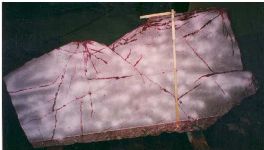
Figure I.9: Crack patterns observed around Ø51mm blast-holes. Saiang (2008).
