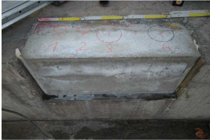
Figure 2.7: Testing block filled with fast hardening cement in front.
