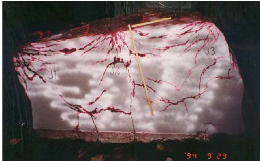
Figure I.10: Crack patterns observed around \varnothing 24\text{mm} blast-holes. Saiang (2008).
