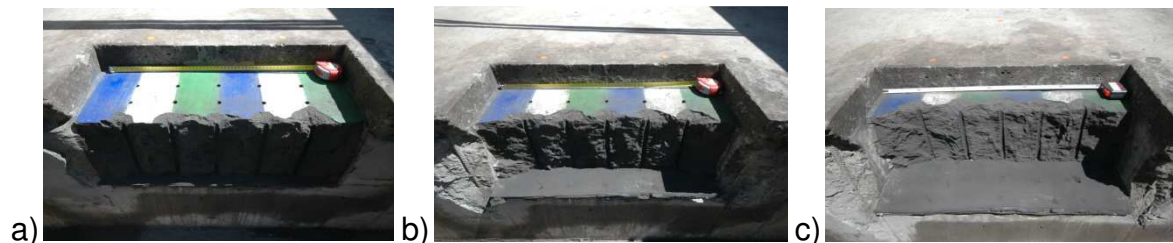
Figure 2.6: Front view after blasting of: a) 1 st row; b) 2 nd row; c) 3 rd row
