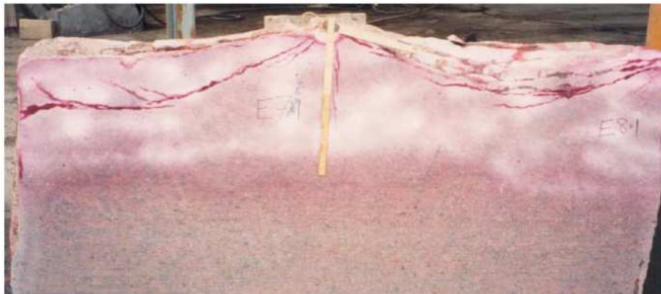
Figure I.8: Bow-shaped tangential cracks. Saiang (2008).
