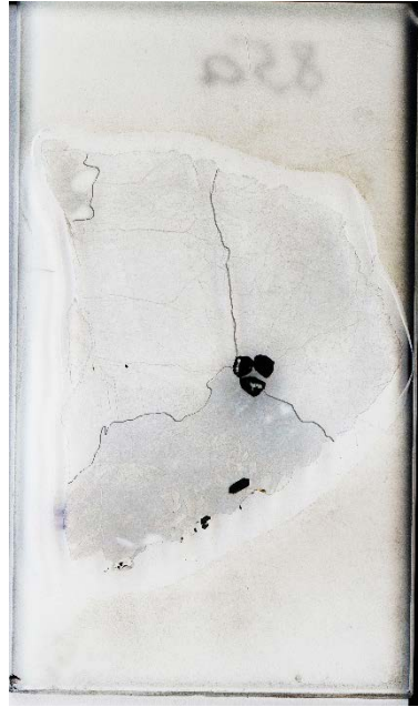
Fig. 54: Scanned thin section 85A with quartz, feldspar and tourmaline (dimensions: 2.8 x 4.8 cm)
