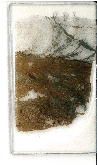
Fig. 92: Scanned thin section 29D with brownish tourmaline, feldspar groundmass (dimensions: 4.8 x 2.8 cm)
