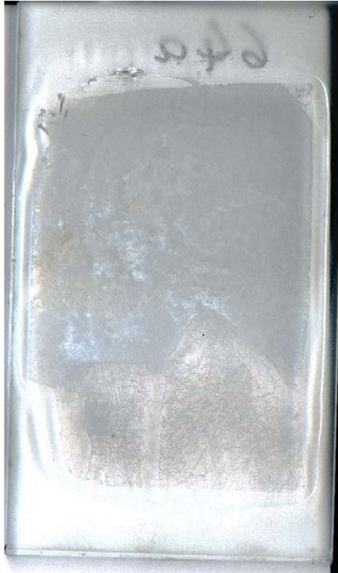
Fig. 39: Scanned thin section 64A with large feldspar crystals at the bottom (dimensions: 2.8 x 4.8 cm)
