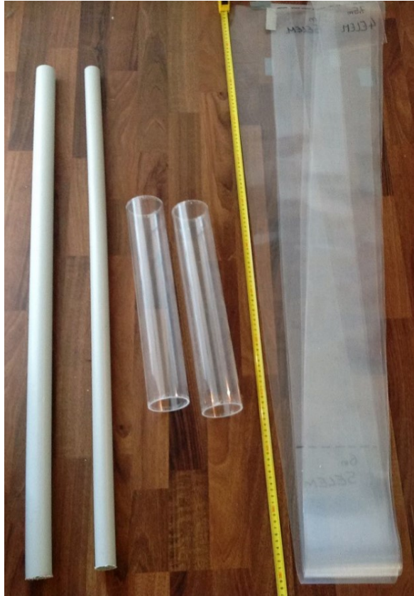
Figure 47: Components used for the inner pipe diameter tests
