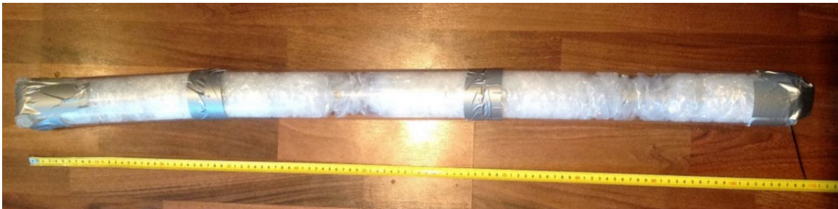
Figure 17: 1 m of protection container filled via the subcomponent folding technique with 16,7 m of plastic hose
