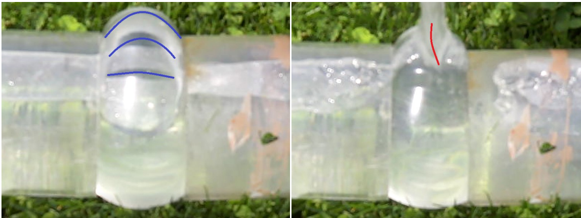
Figure 27: Comparison of stretch marks (blue) to rupture (red) direction, in a 4,5 cm gap under 4,4 bar pressure
