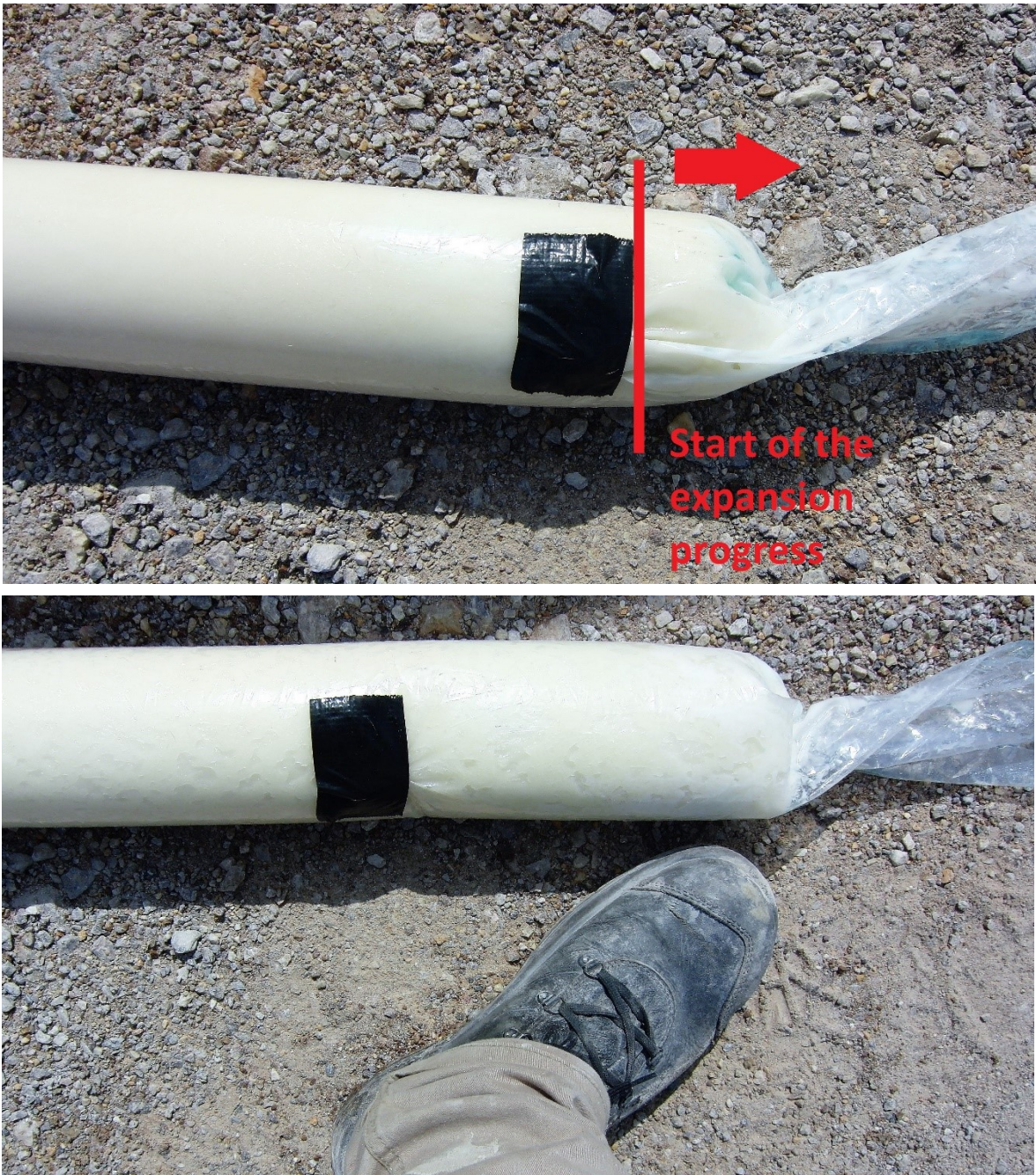
Figure 56: Strat (top) and finish (bottom) of matrix expansion inside a 3 m long plastic hose
