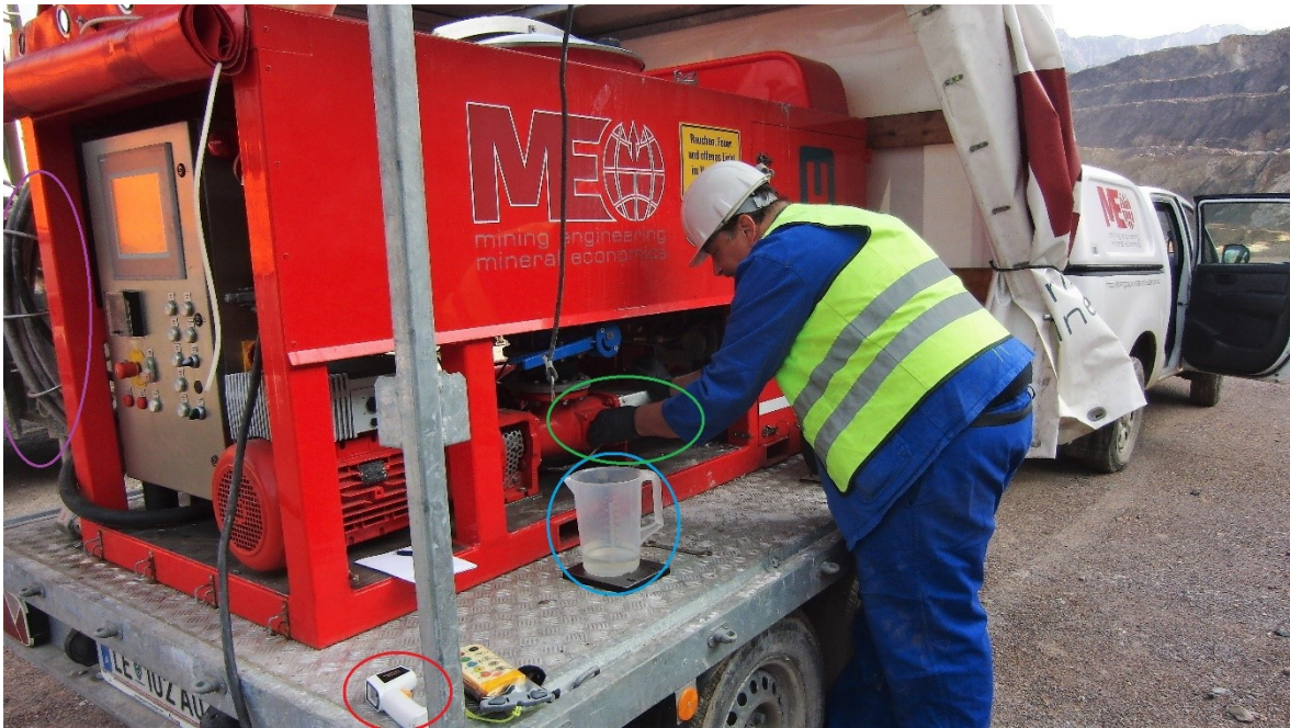
Figure 3: Controlling of the MUL-BBK emulsion pumping unit
