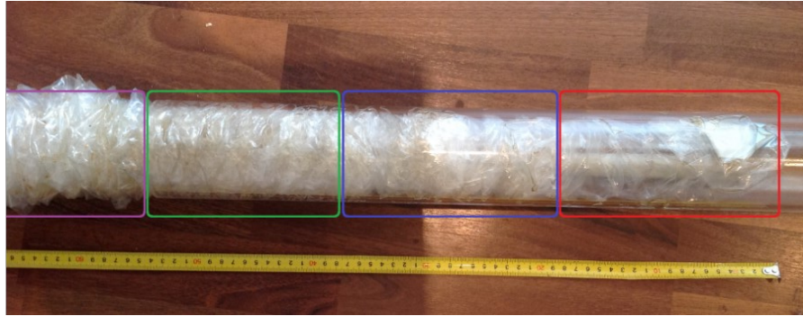
Figure 11: Cramming via folded windings technique using a protection container with a diameter of 80/75 mm
