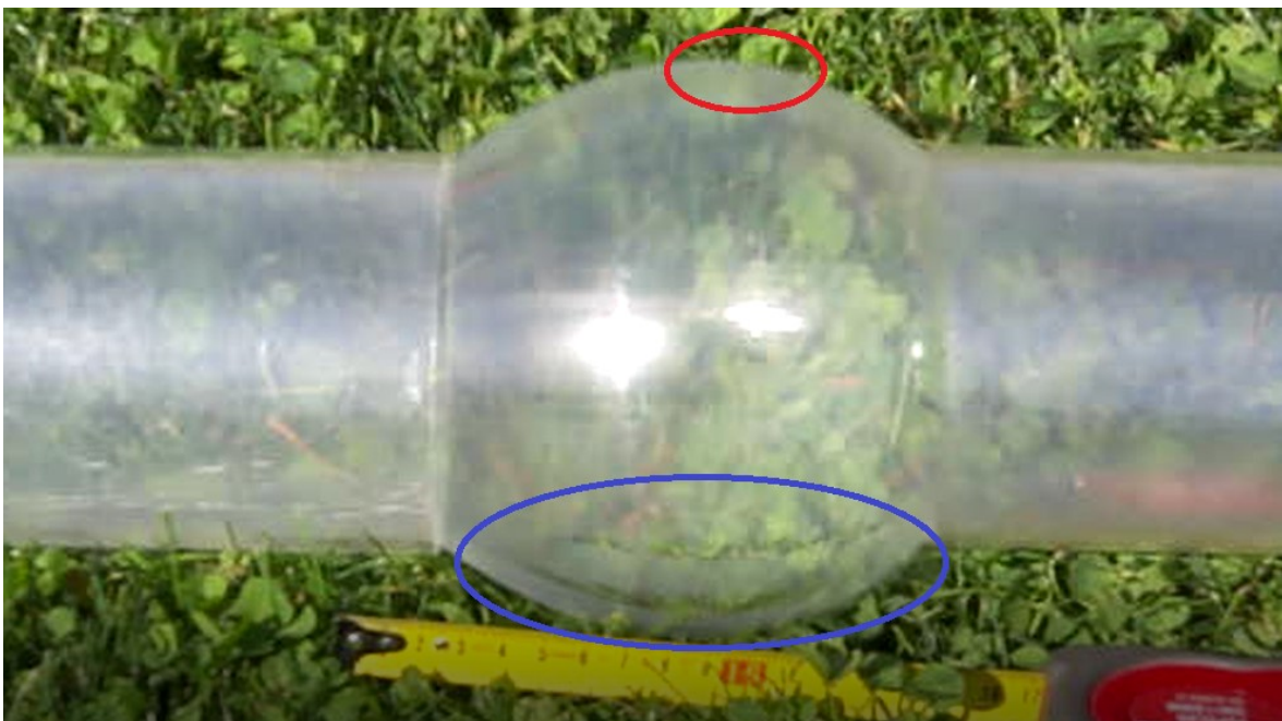
Figure 24: Plastic hose between a 12 cm gap influenced by 0,9 bar briefly before the point of failure occurs
