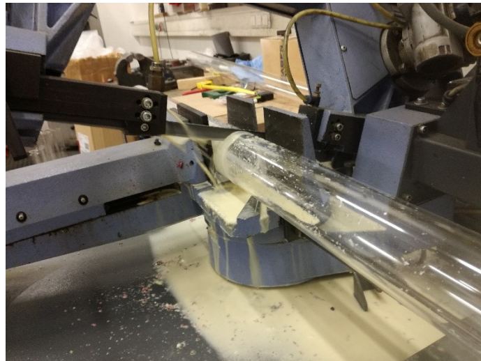
Figure 29: Automatic metal cutting saw, supported by an oil-water blend
