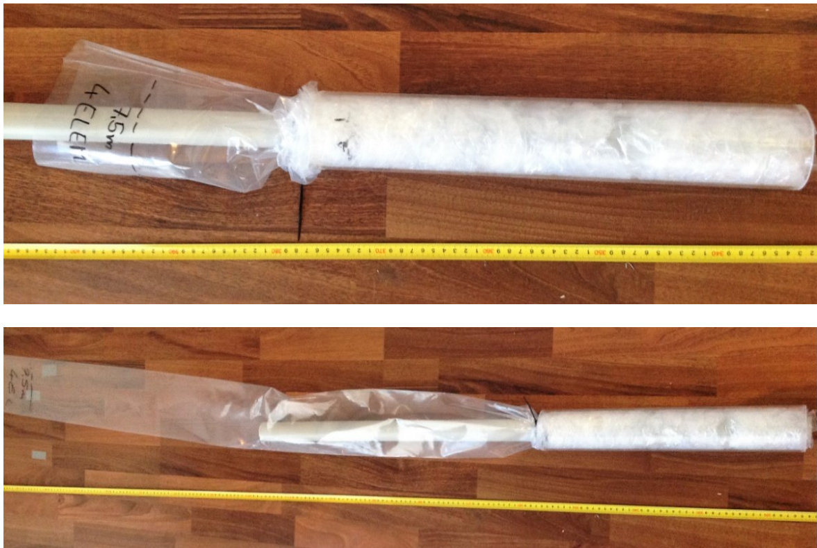
Figure 48: Comparison of storage possibilities using a 32 mm diameter inner pipe (top) and a 45 mm inner pipe (bottom)
