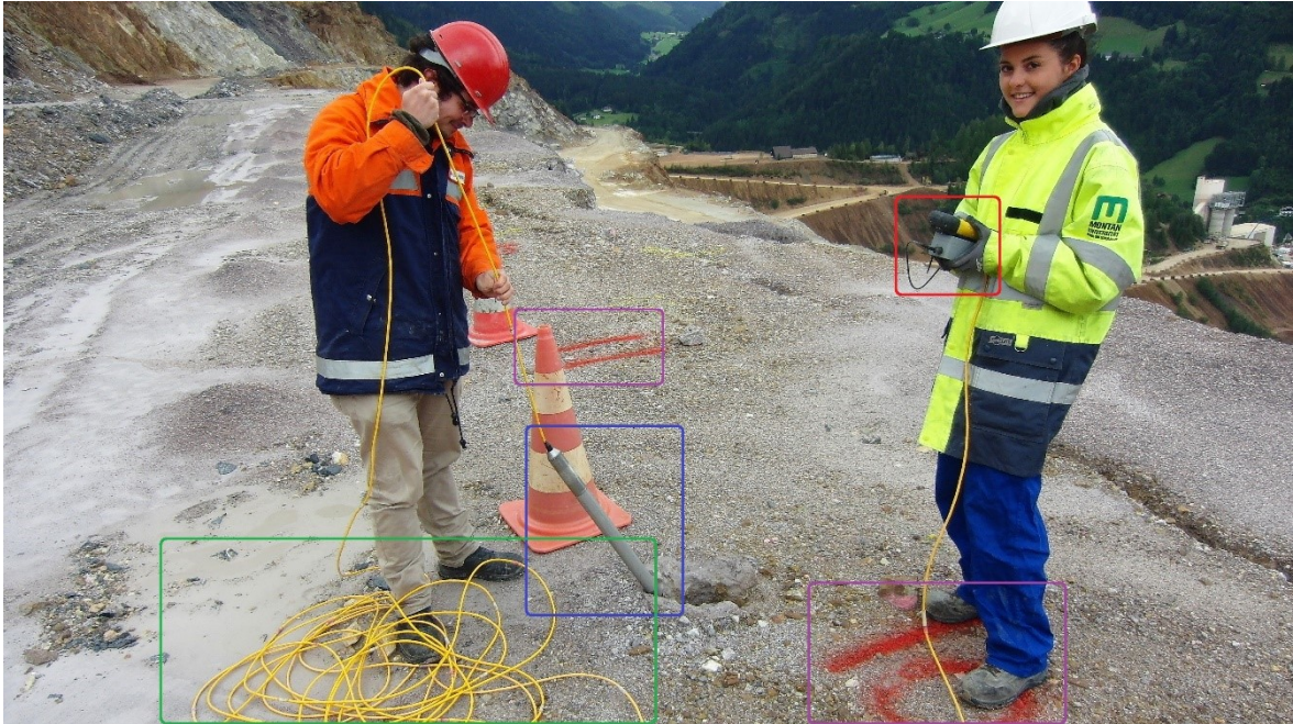
Figure 38: Deployment of the Pulsar probe
