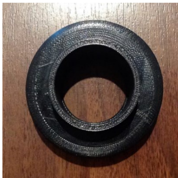
Figure 50: Unfolding device made out of PLA material
