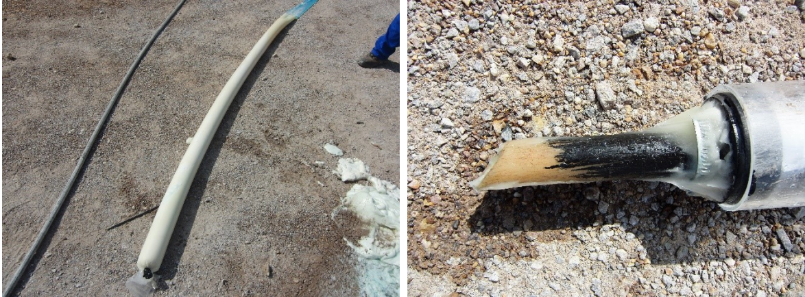
Figure 55: Summary of the connection test between charging hose and prototype
