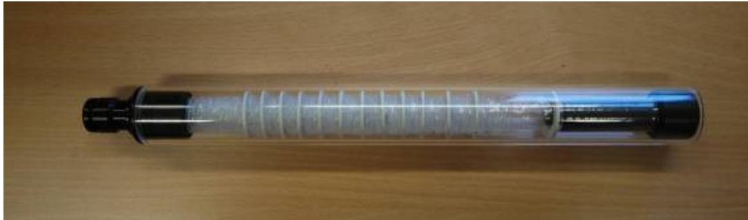
Figure 2: ContBlast Charging Unit ready for filling (Source: Ivanova)
