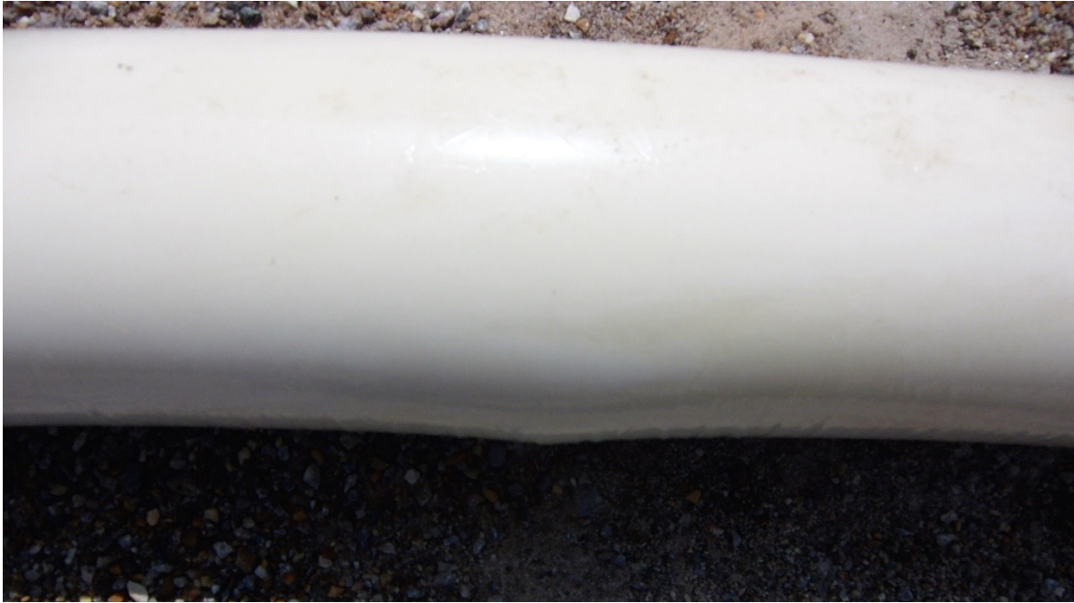
Figure 57: Protrusion near the one-meter mark, starting from the closed part of the hose
