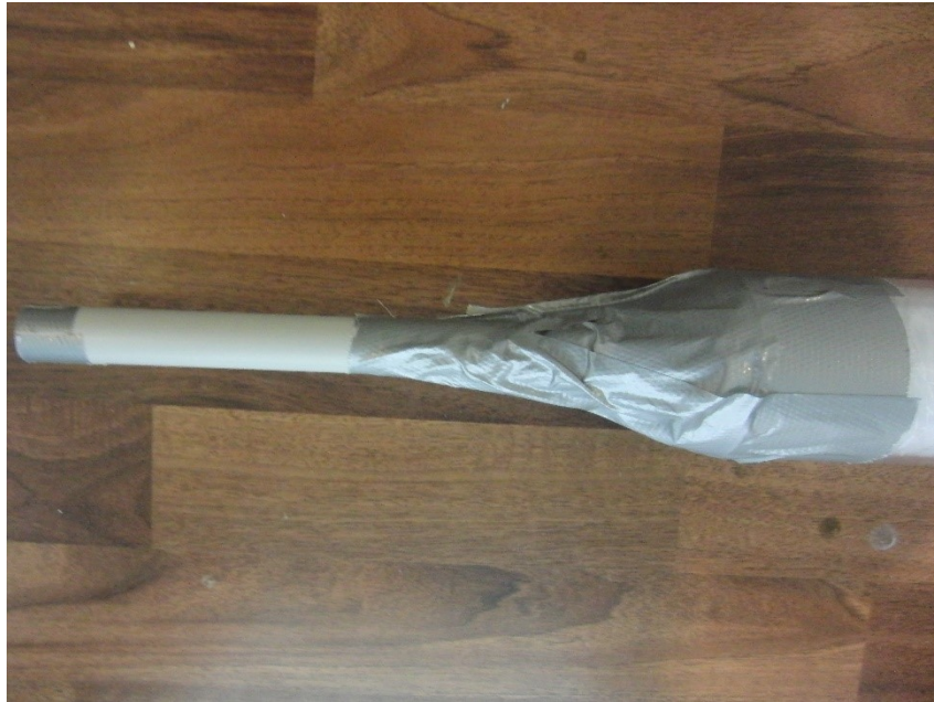
Figure 34: Cylindrical connection between inner pipe and protection container formed by Duct Tape
