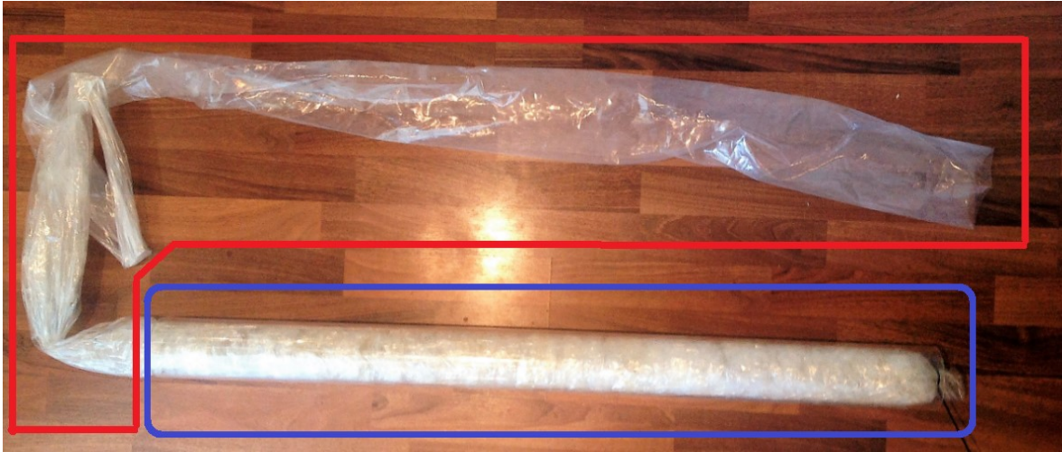
Figure 12: Using a wrapper to force the plastic hose through the protection container
