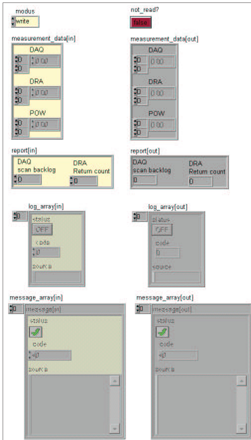
Figure 156: Front Panel of TSUL_TemporaryStorage_UserInterface.vi
