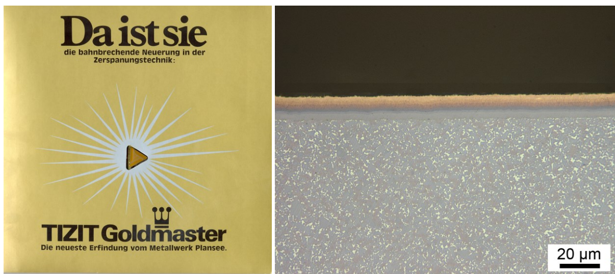
Fig. 7: Goldmaster GM35 coating, total thickness of 12 µm with a coating architecture of TiC, four layers TiCN, with increasing nitrogen content and TiN, introduced in 1973 [51].
