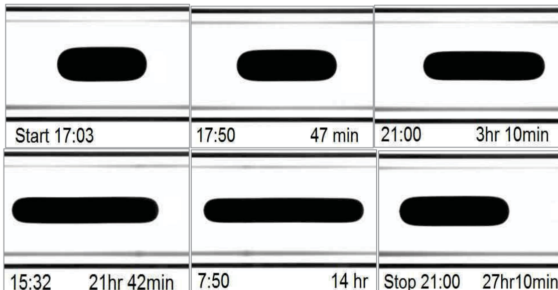
Figure 66: Transformation and motion of the oil droplet over time (starting top left corner). Oil sample -"Crude oil A". Rotational speed - 5000 \text{ min}^{-1}
