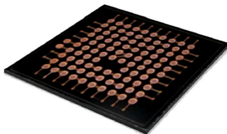
Figure 3: The semiconductor silicon die with copper-patterned side [9].
