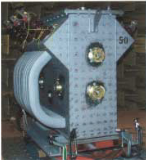
Fig. 5.2: The test transformer in the anechoic room
