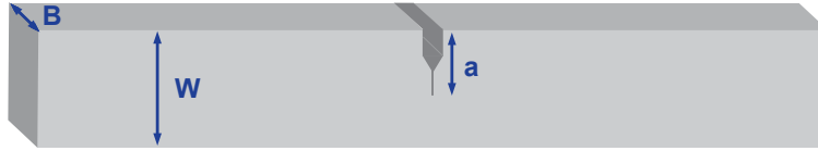
Figure A.4: Illustration of relevant sample dimensions at the example of an SENB specimen
