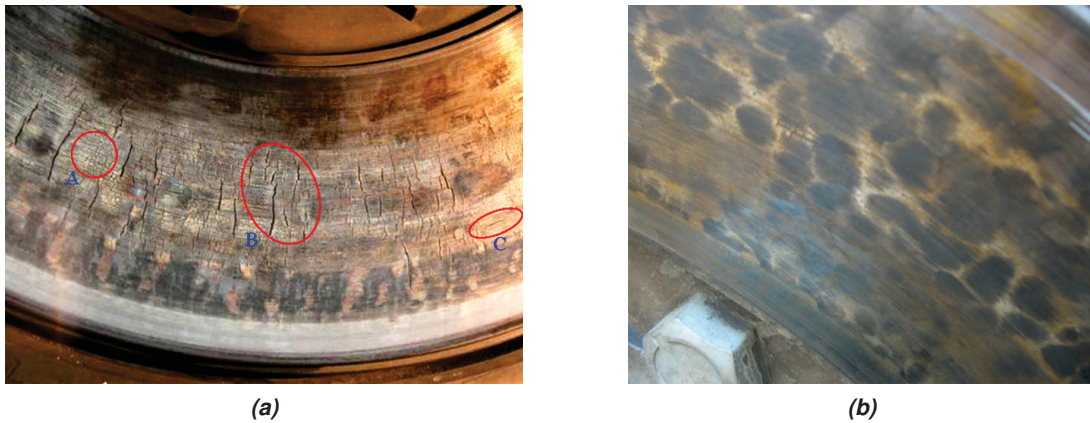
Figure 1.6: a) Cracks at the friction surface: A) network of small cracks, B) radial crack, C) tangential crack and b) Hot spot pattern after braking [4].
