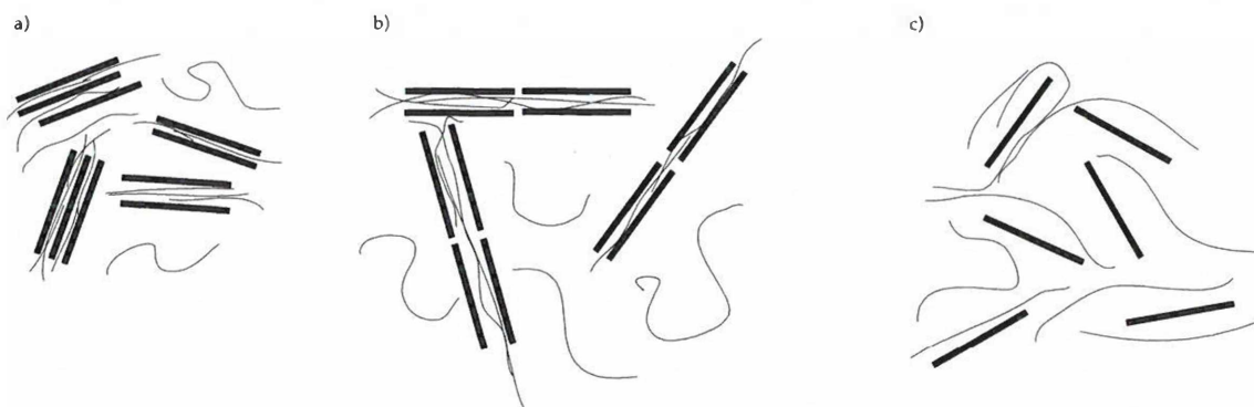
Figure 2.13: Different types of OMLS incorporation into the polymer. a) intercalation b) intercalation with flocculation c) exfoliation
