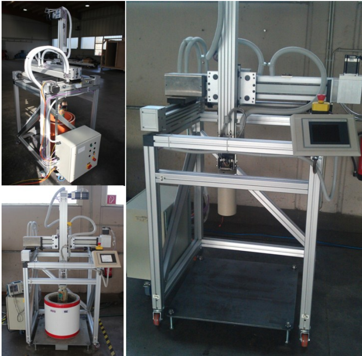
Figure 4-1. Test robot used to simulate drill string movement
