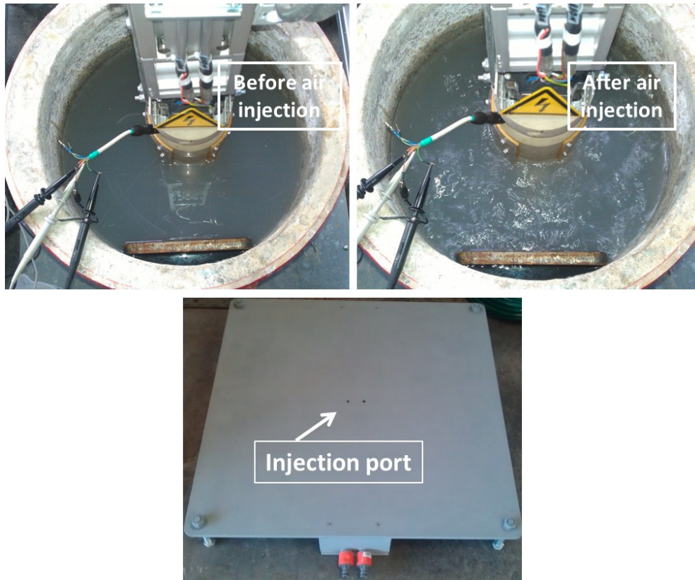
Figure 4-43. Wellbore condition before and after air injection to the water
