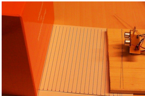
Figure 4-9. Testing for the blind zone area
