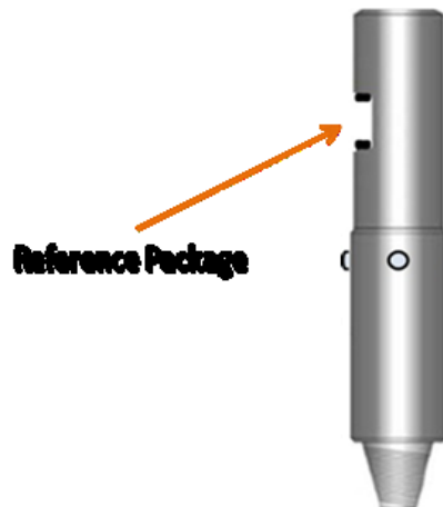
Figure 5-1. Referenced ultrasonic sensor, measures the speed of sound in mud at different Pressure and temperature
