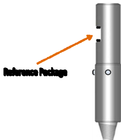
Figure 4-4. Referenced package, measures speed of sound in mud at different Pressure and temperature
