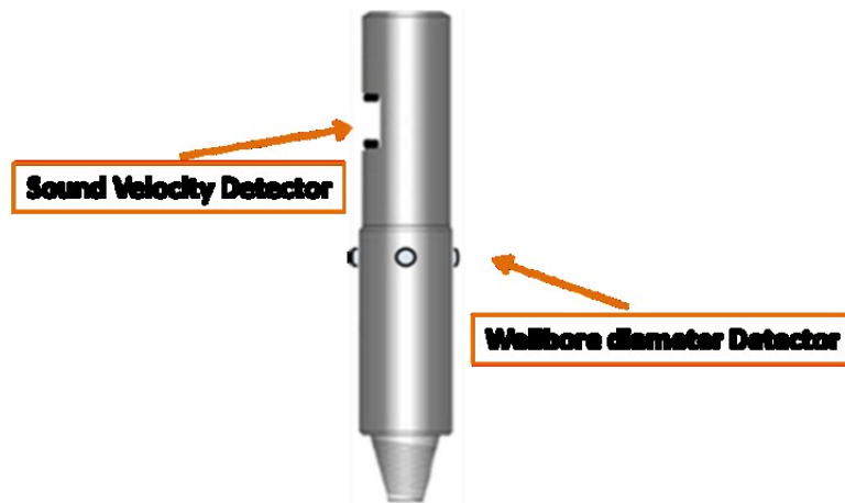
Figure 4-42. Ultrasonic caliper sub
