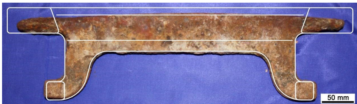
Fig. 6: Comparison of worn grate bar with the technical drawing (white lines)
