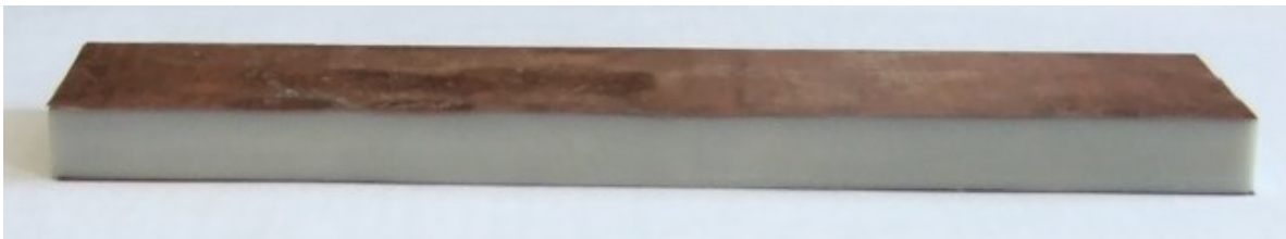
Fig. 2. Specimen for the cyclic four point bend tests
