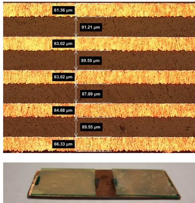
Fig. 3. Specimen for the cyclic tensile-compression tests.
