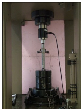
FIGURE 95: ROCK TESTING MACHINE AND DDS
