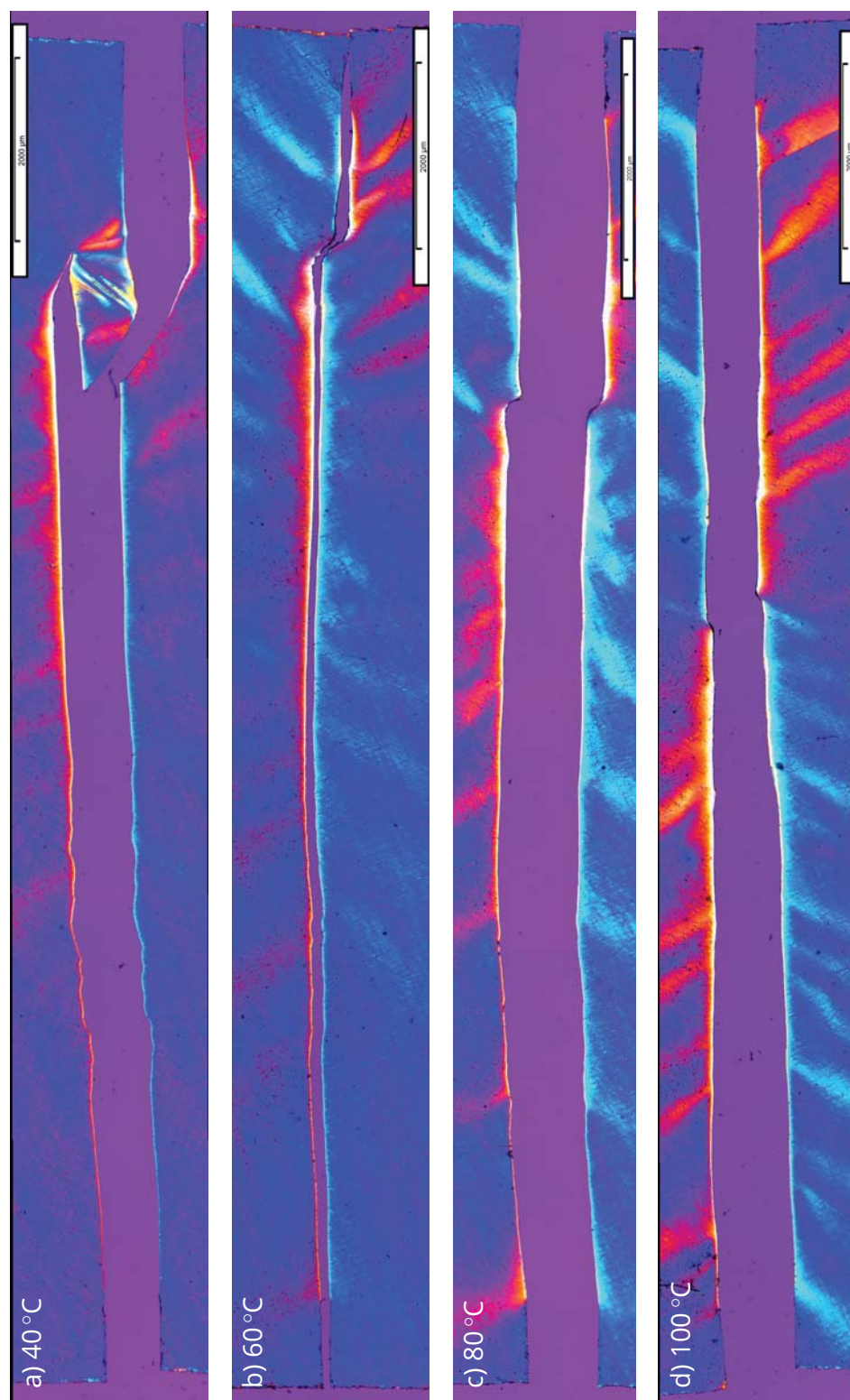
Figure 3.37: Polarized light microscopic images of fracture surfaces from temperature dependent fatigue tests with 1L 4.5 -PET(C) 4.5 at a) 40 °C, b) 60 °C, c) 80 °C and d) 100 °C.
