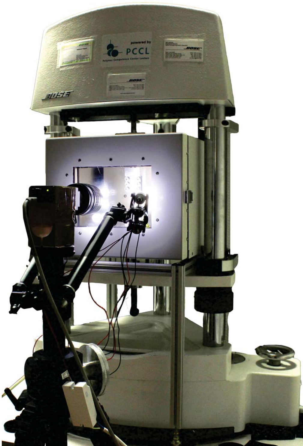
Figure 3.15: Fatigue test setup consisting of an electrically driven fatigue test machine Bose 3230 with special unperforated lightweight aluminum clamps, an optical system Pixelink B959 and high output LEDs.
