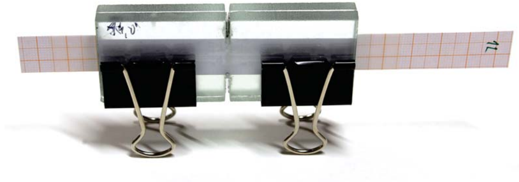
Figure 3.9: Templates made of glass for the preparation of DENT specimens with a defined crack length of 0.5 mm.
