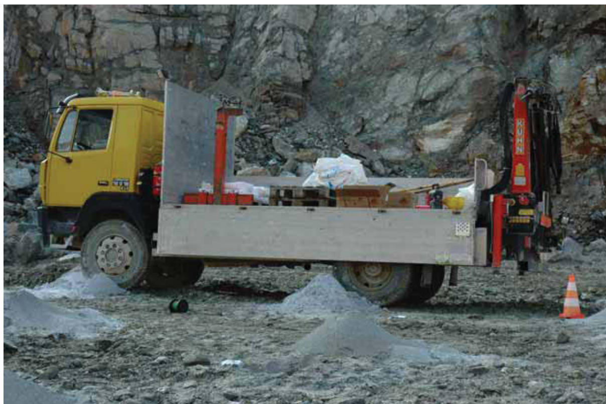
Figure 3: The blasters truck with the crane mounted to it
