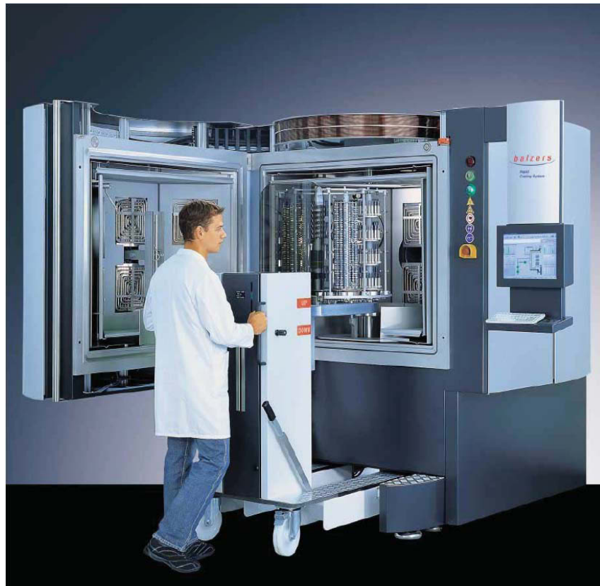
Figure 5.1: Balzers RCS industrial scale cathodic arc evaporation facility [61]
