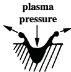
Figure 2.4: Particle formation at cathode spots [12]
