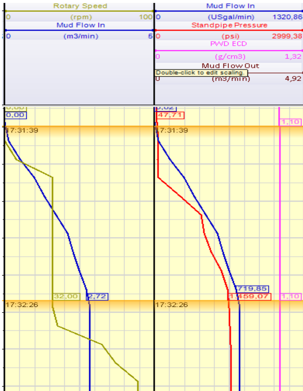
Figure 23. Pump Start-up Type 1
