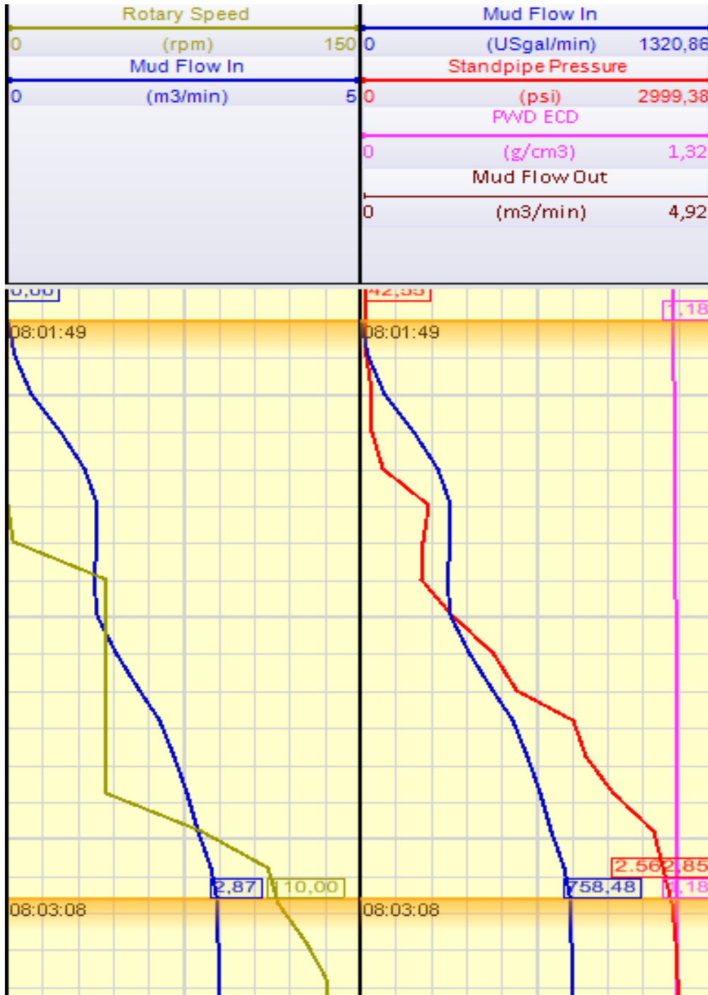
Figure 24. Pump Start-up Type 2
